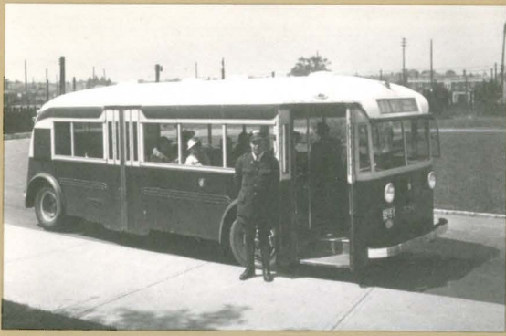
1937: A radical advance when the TTC took delivery of the first rear-engined buses with reduced noise and vibration and easier handling characteristics. By 1940, 82 were in use.
