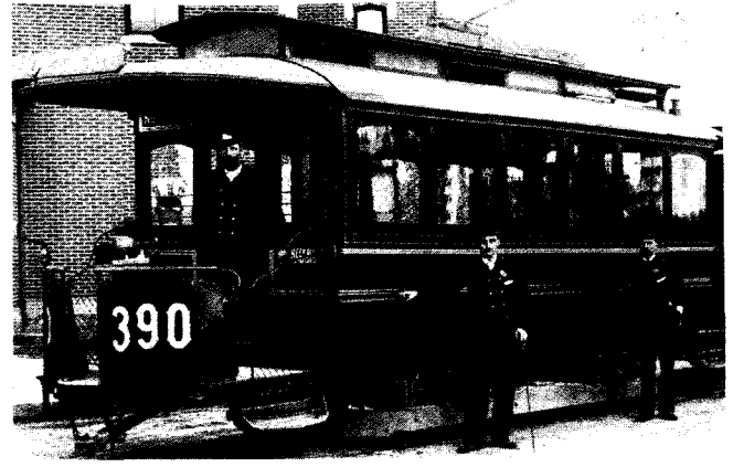
One of the first electric street cars built between 1892 and 1894 by the Toronto Railway Co. (TRC) to replace horse cars.
