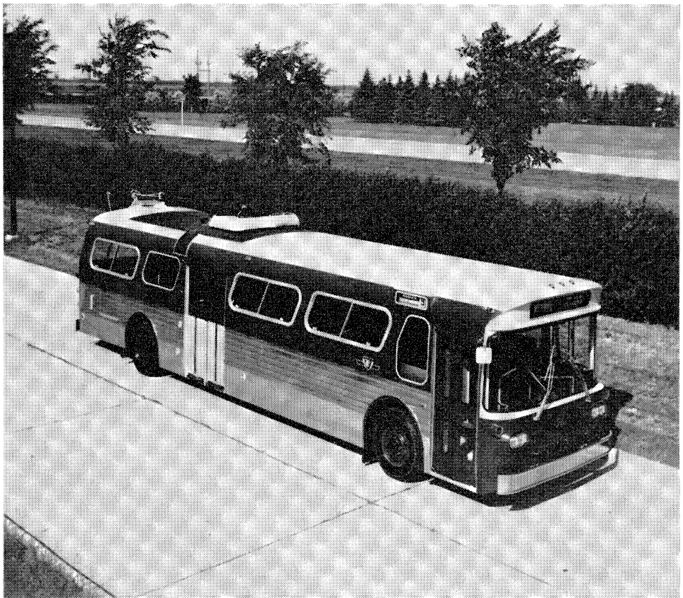
A new look for an old TTC trolley bus. This is the first of two test trolley buses to have completely new bodies designed around the traction motors, control equipment and other electrical components taken from trolley buses from the existing fleet. The new vehicle shown above was rebuilt in Winnipeg. A second vehicle is being rebuilt in England.
