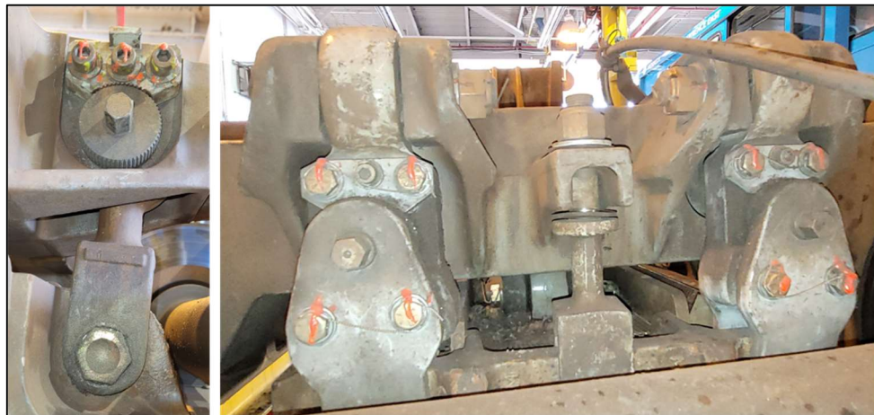
Figure 83 - Vertical Connection Links on Truck S/N 027
