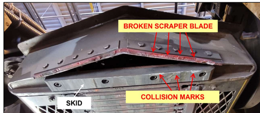
Figure 80 - Scraper Blades and Skid Damage on Truck S/N 027
