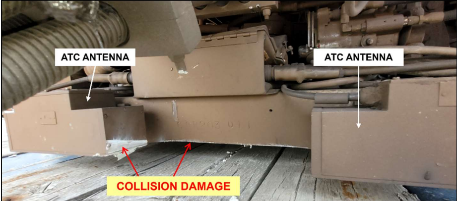
Figure 74 - Preliminary Damage Assessment on Truck S/N 027
