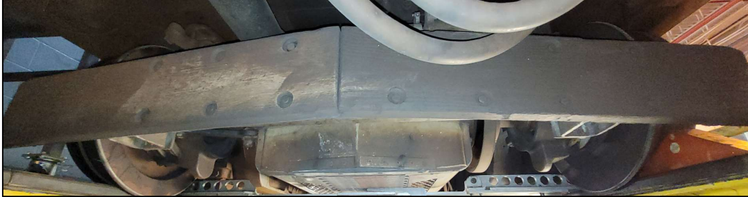
Figure 64 - Safety Fender on Truck S/N 005
