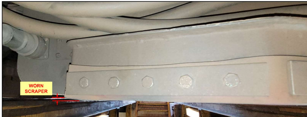
Figure 36 - Worn Scraper Blade
