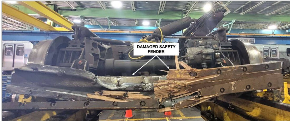
Figure 95 - Damaged Safety Fender
