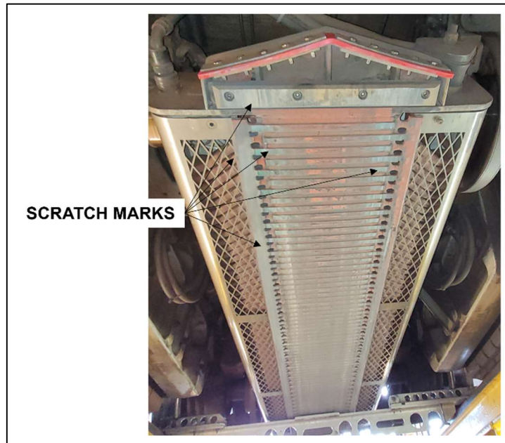
Figure 136 - Scratch Marks on Bottom of the LIM
