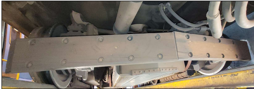
Figure 119 - Safety Fender on Truck S/N 009
