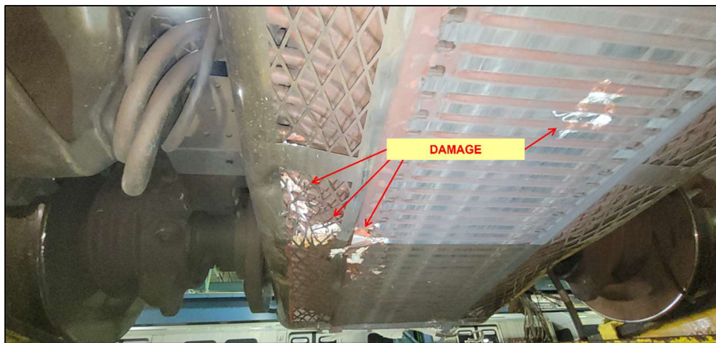
Figure 92 - LIM bottom damage
