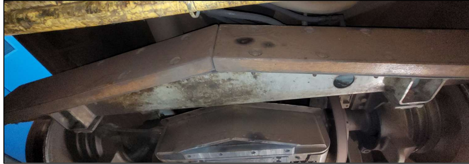
Figure 58 - Safety Fender on Truck S/N 028
