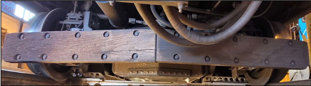
Figure 103 - Safety Fender on Truck S/N 021
