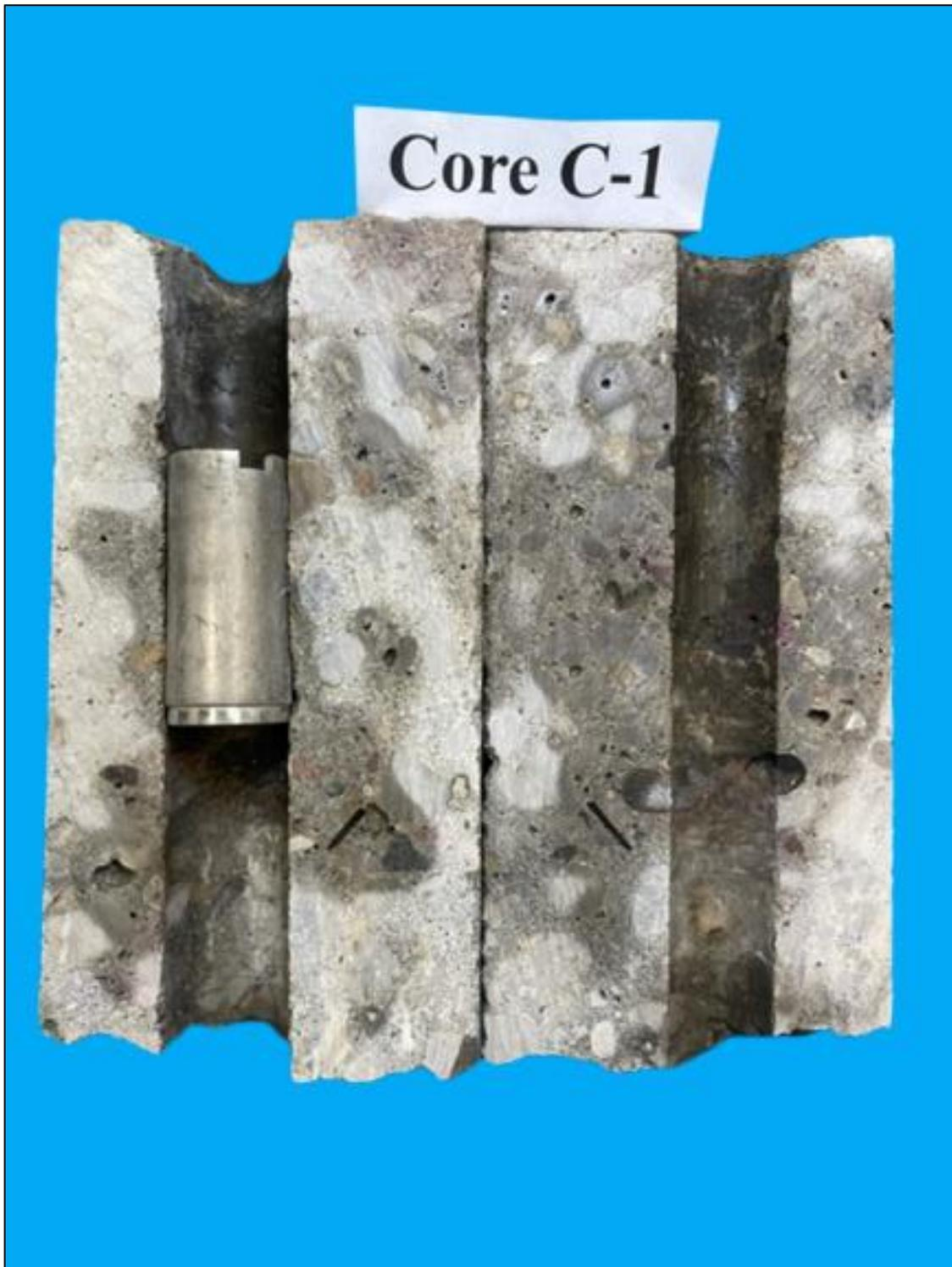
Photo P2 – Core C1 Sawn Sample Faces
