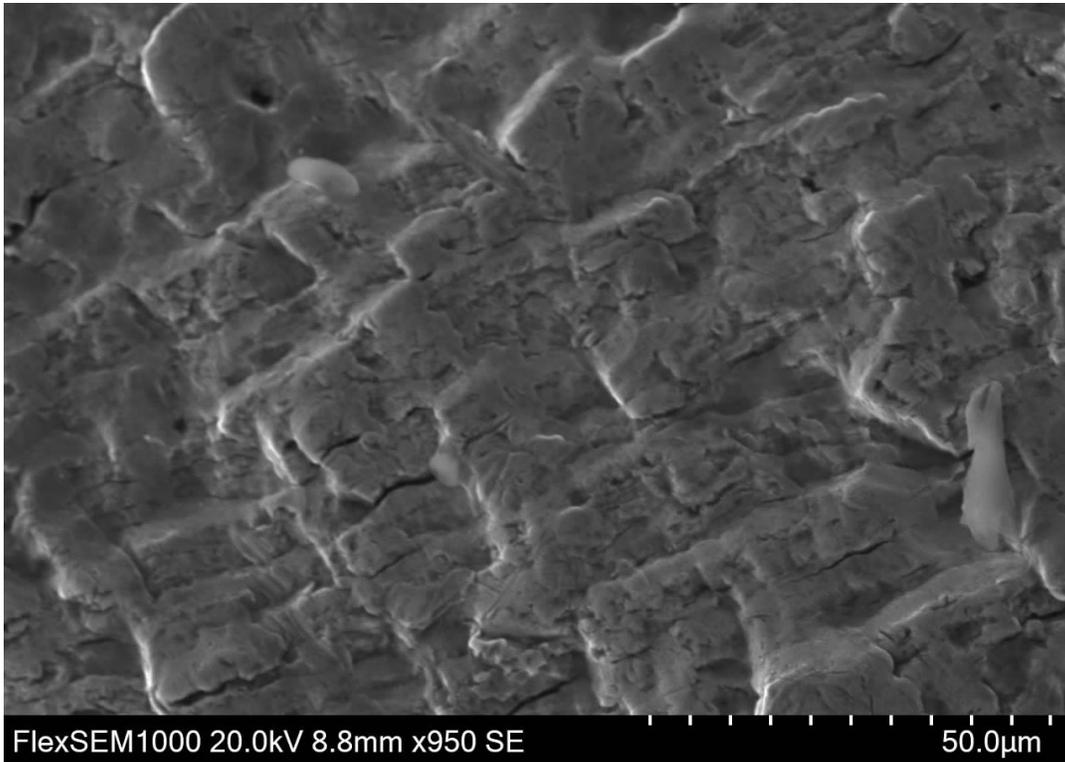
**FIGURE 40. CLOSER VIEW OF BURNISHED FRACTURE FEATURES 12 O'CLOCK REGION, BOLT C2**
