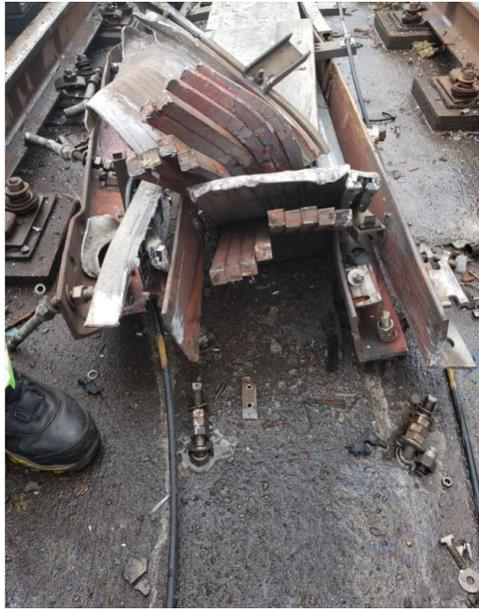
*Figure 8: Front of Incident Reaction Rail Assembly*
