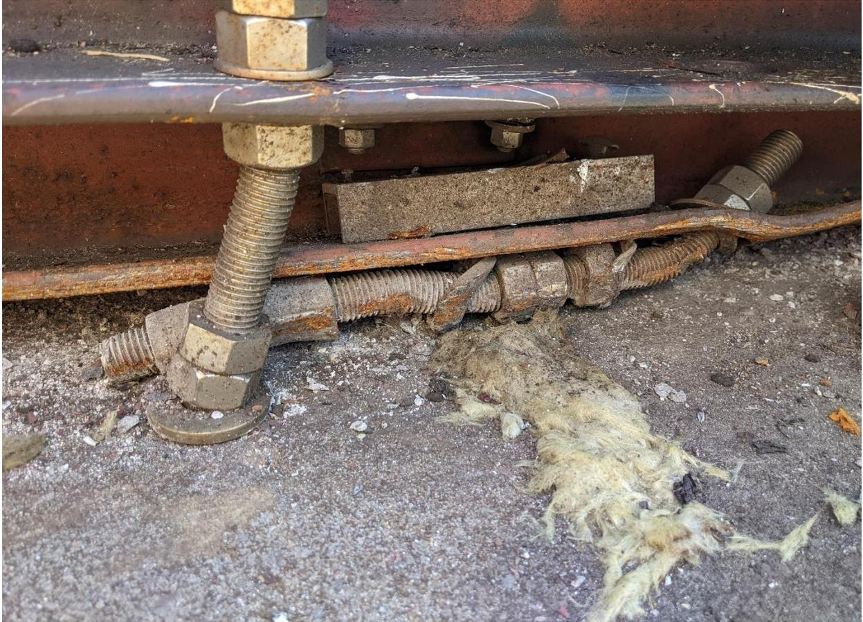
*Figure 15: Upper Portion of Anchor Bolt Attached to Reaction Rail Frame (Anchor No. 7). Note that the spacer sleeve remains attached to rod, while cone and expansion sleeve remained within the concrete.*
