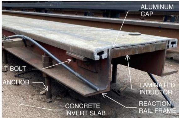
Figure 16: Typical Reaction Rail Components
