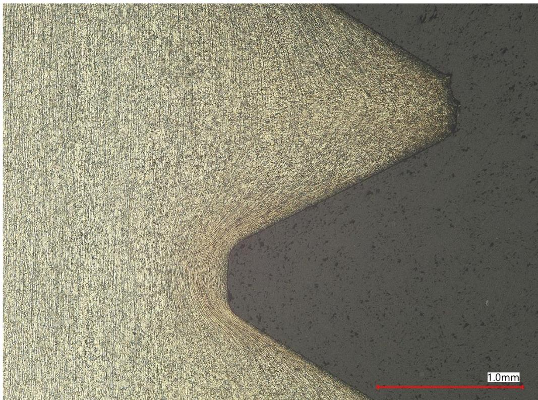
**FIGURE 56. FLOW LINES ON THE THREADS, BOLT C2**
