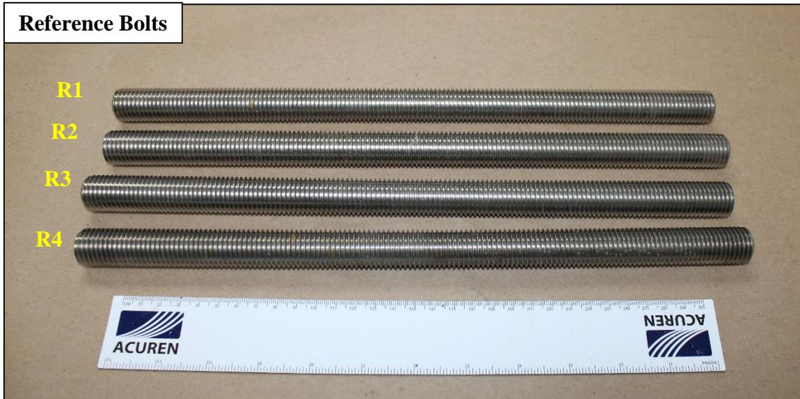
**FIGURE 15. PHOTO OF THE REFERENCE BOLTS AFTER REMOVING HARDWARE.**
