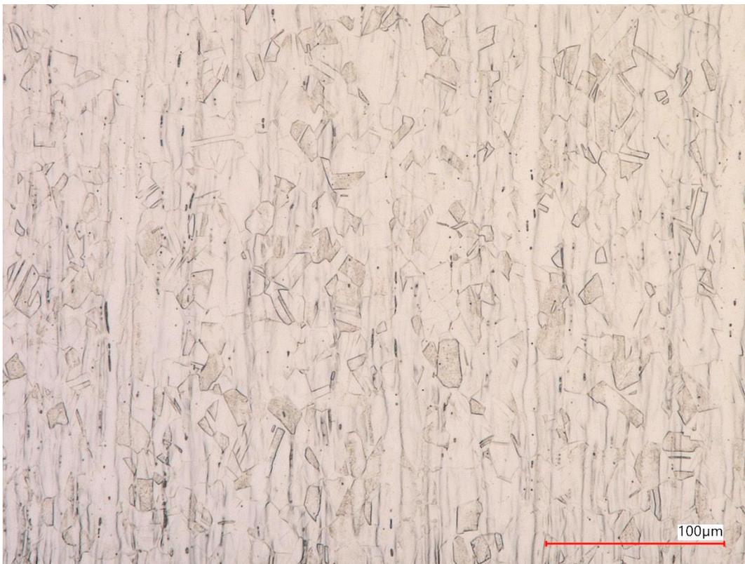
**FIGURE 72. CORE MICROSTRUCTURE OF BOLT R1**
