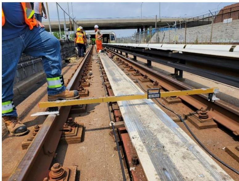
*Figure 12: Cross-level, combination track gauge used for track inspection, and TOR-Reaction rail elevation measurements taken at a joint south (southbound) of derailment site.*
