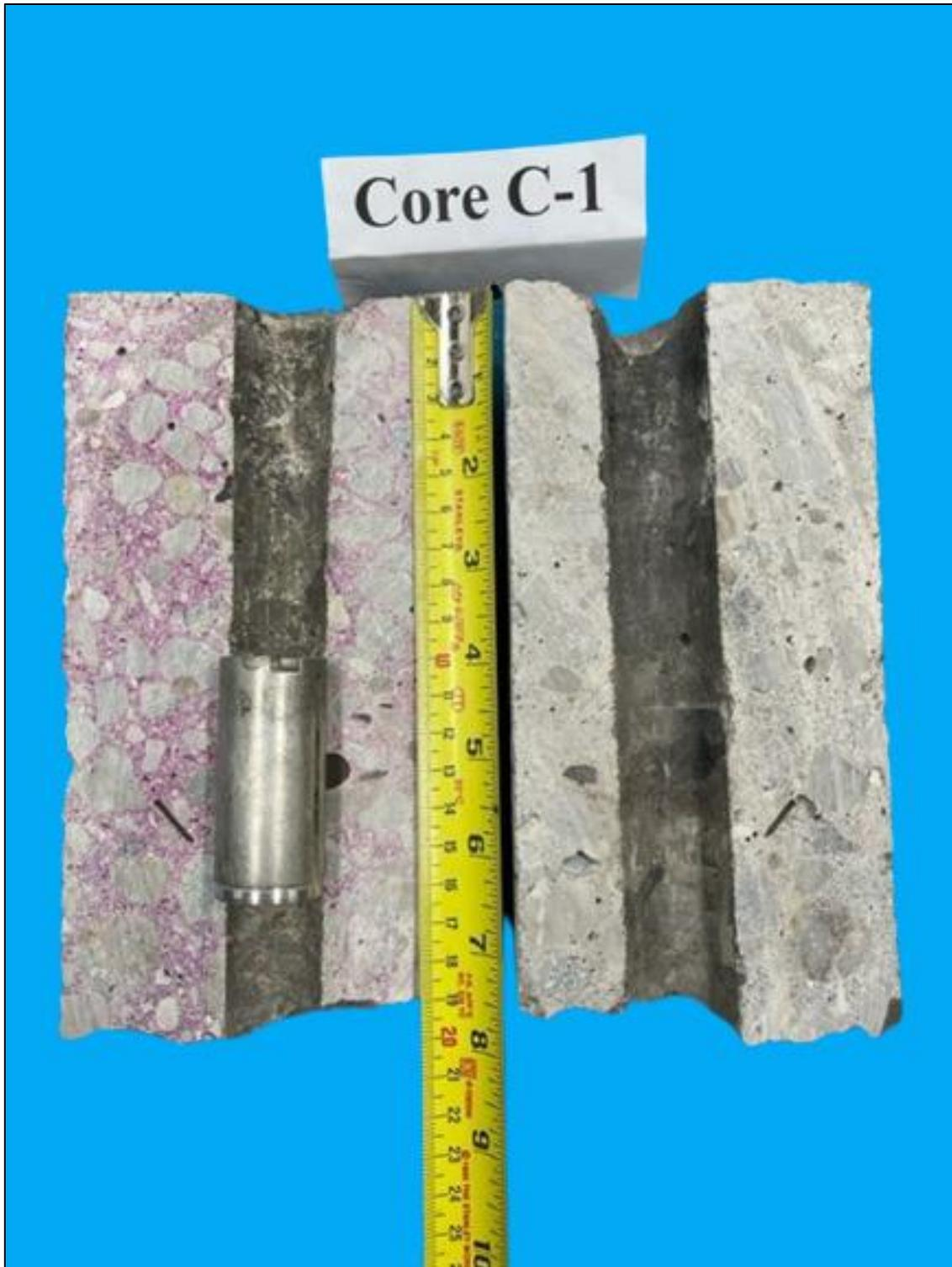
**Photo P3 –Core C1 Sawn Sample Faces**
