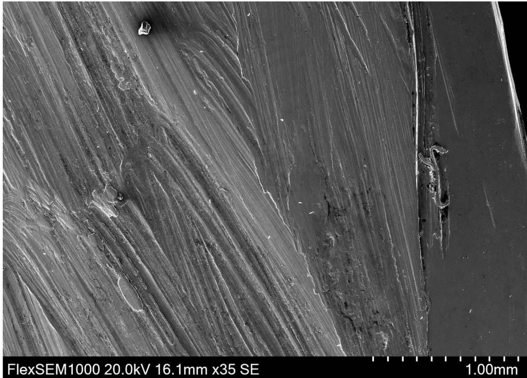
**FIGURE 50. HEAVY SCRATCH MARKS ON THE FRACTURE SURFACE, ANOTHER AREA, BOLT C5**
