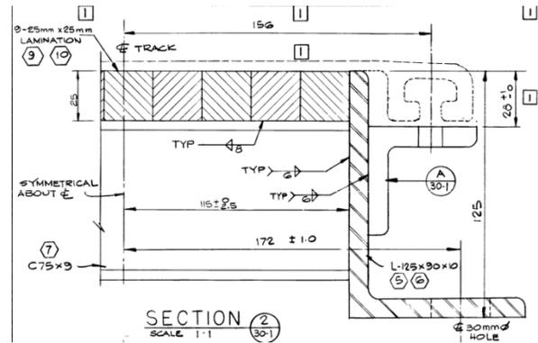
Figure 17: Typical Reaction Rail Drawing - Section
