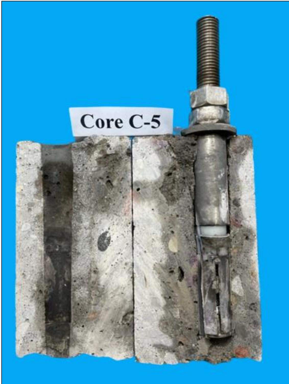
Photo P21 – Core C5 Sawn Sample Faces
