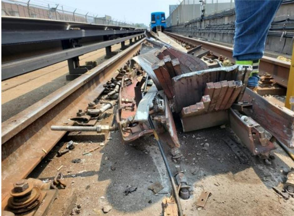
*Figure 2: Section of Reaction Rail which came in contact with Linear Induction Motor*
