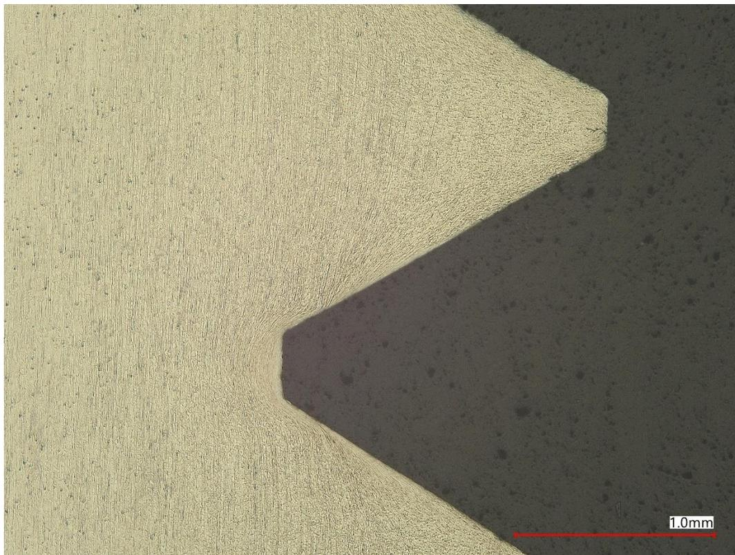
**FIGURE 74. FLOW LINES ON THREADS, BOLT R2**
