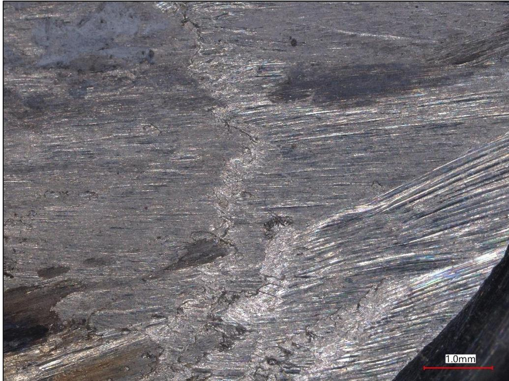
**FIGURE 27. CLOSE VIEW OF SCRATCH MARKS ON FRACTURE SURFACE, BOLT C5**
