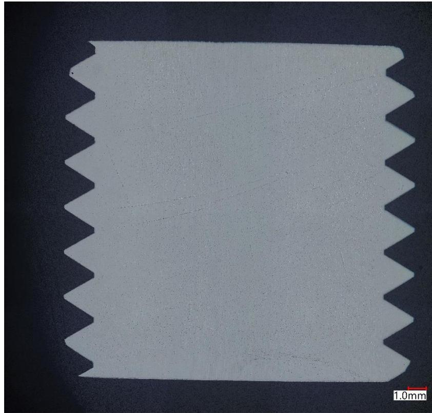
**FIGURE 81. GENERAL IMAGE OF BOLT R4 IN AS-POLISHED CONDITION**
