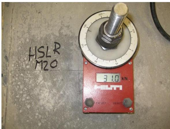
Figure 25: Post-Installed Anchor Test
