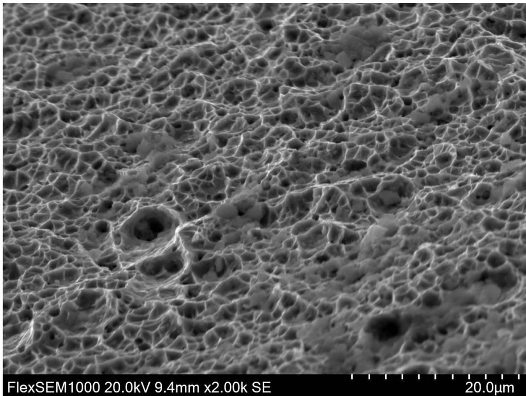
**FIGURE 45. CLOSER VIEW OF AREA MARKED “FINAL FRACTURE” IN FIGURE 43, BOLT C2**
