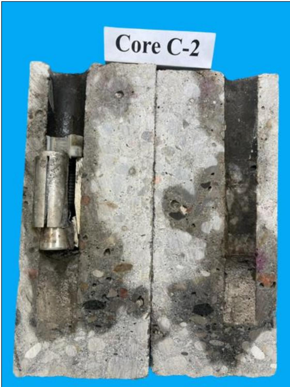
**Photo P7 – Core C2 Sawn Sample Faces**
