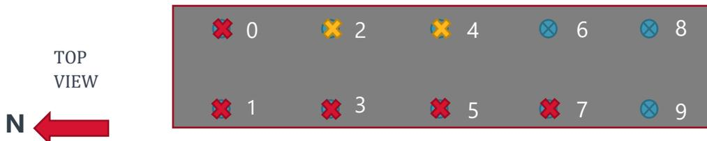
*Figure 34: Plan view of suspected bolt failures. Red represents confirmed failed anchor bolts, and yellow represents suspected loose anchor bolts*
