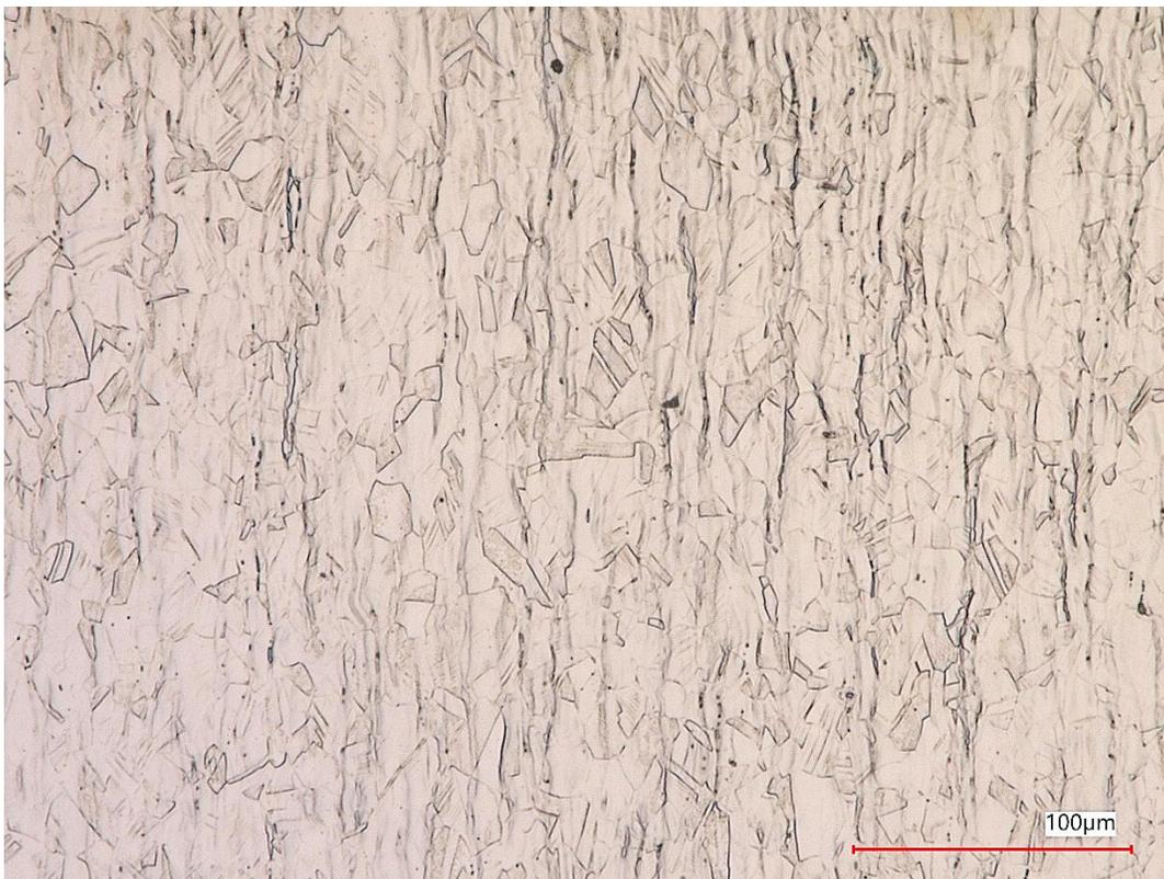
**FIGURE 80. CORE MICROSTRUCTURE OF BOLT R3**
