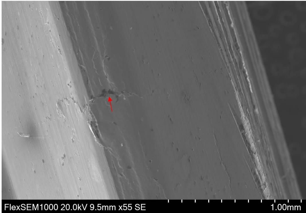
**FIGURE 46. ONE OF THE CRACKS LIKE INDICATIONS OBSERVED DURING VISUAL EXAMINATION, BOLT C2**
