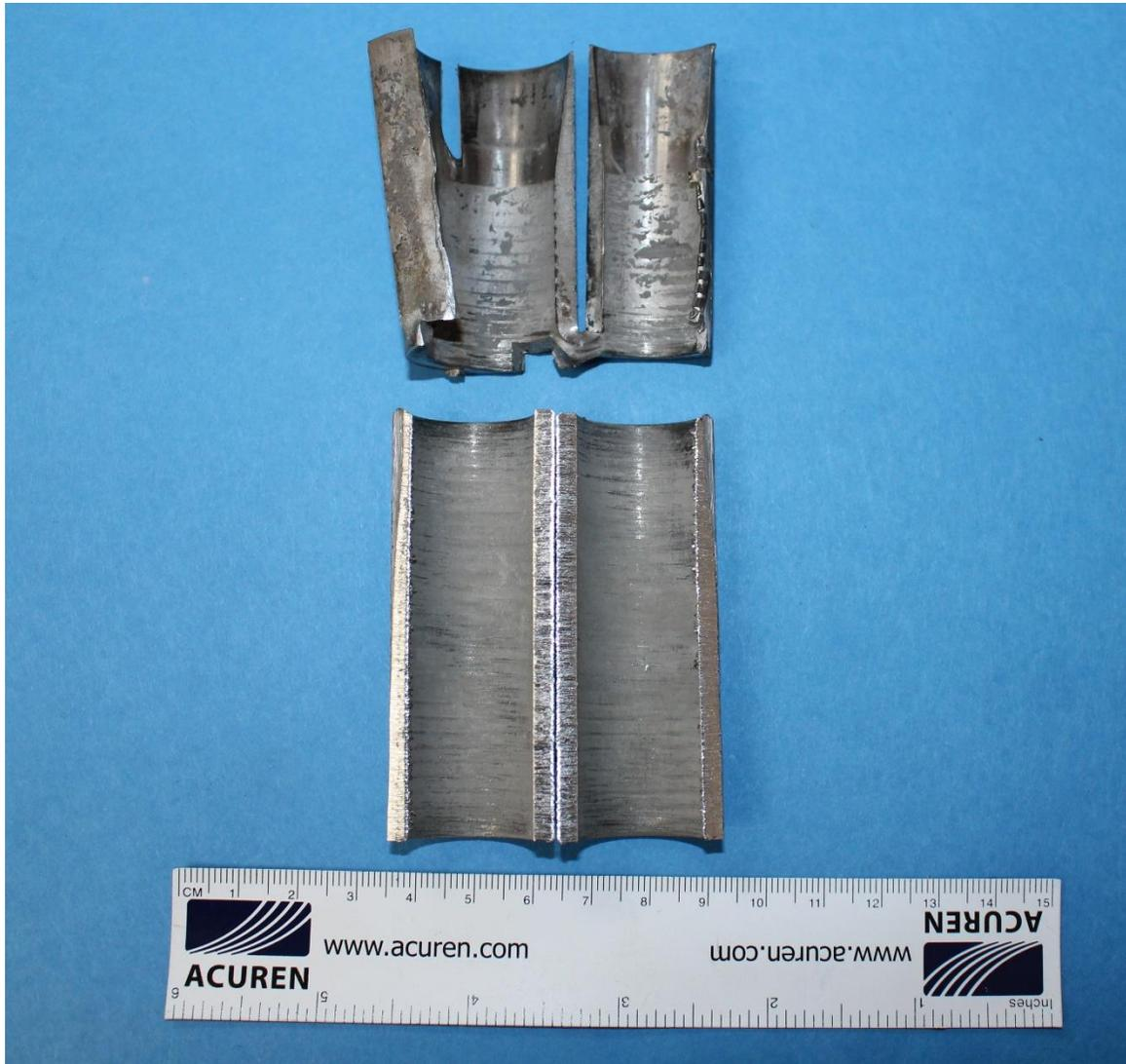
**FIGURE 12. PHOTO OF THE INNER SURFACE OF THE SLEEVE AFTER REMOVING BOLT C5.**
