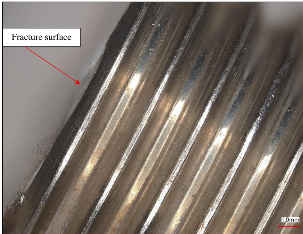
**FIGURE 28. THREADS IN THE VICINITY OF THE FRACTURE SURFACE, BOLT C5**
