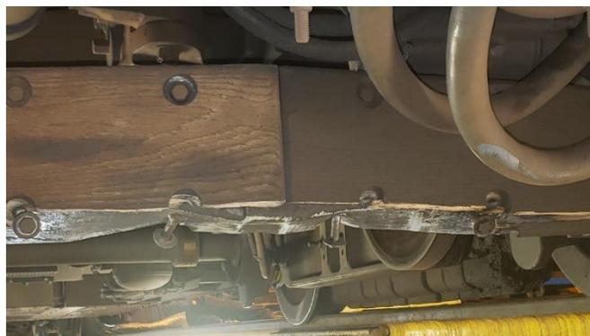
Figure 4: Leading Edge Damage to Truck Fender on car 3006
