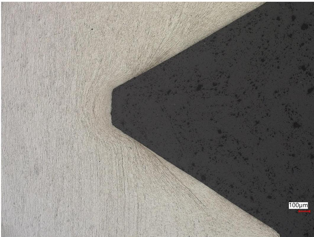
**FIGURE 70. ROOT SHAPE OF THREADS IN BOLT R1, SHARP CORNER**
