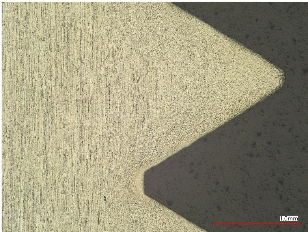
**FIGURE 82. FLOW LINES ON THREADS, BOLT R4**
