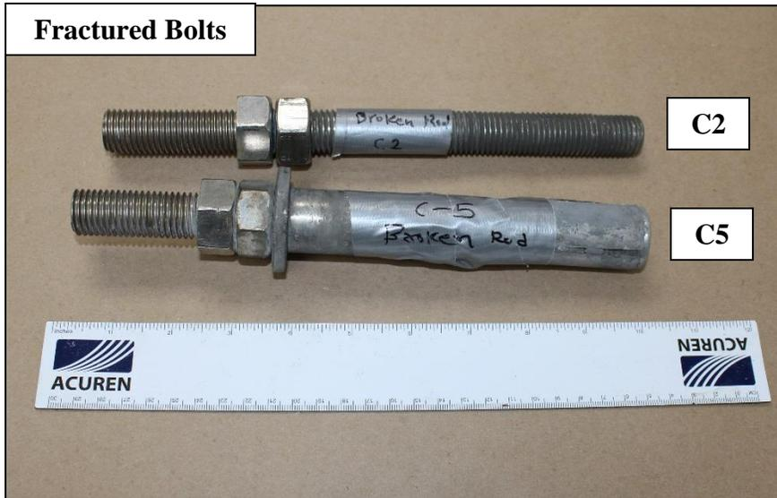
**FIGURE 4. PHOTO OF SUBMITTED FRACTURED BOLTS.**
