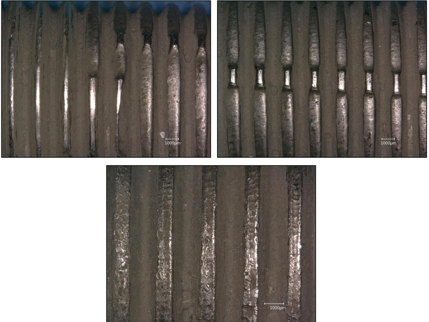
**FIGURE 7. IMAGES SHOWING FEATURES OBSERVED AT AREAS OF STRIPPED THREADS ON BOLT C2.**
