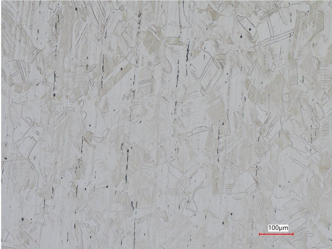
**FIGURE 65. CORE MICROSTRUCTURE, BOLT O1**
