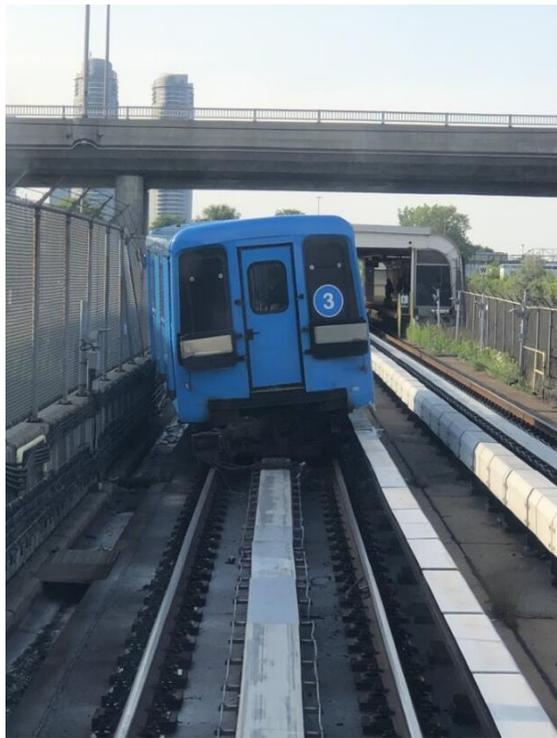
*Figure 1: Derailed consist south of Ellesmere Station taken the evening of July 24<sup>th</sup>, 2023*
