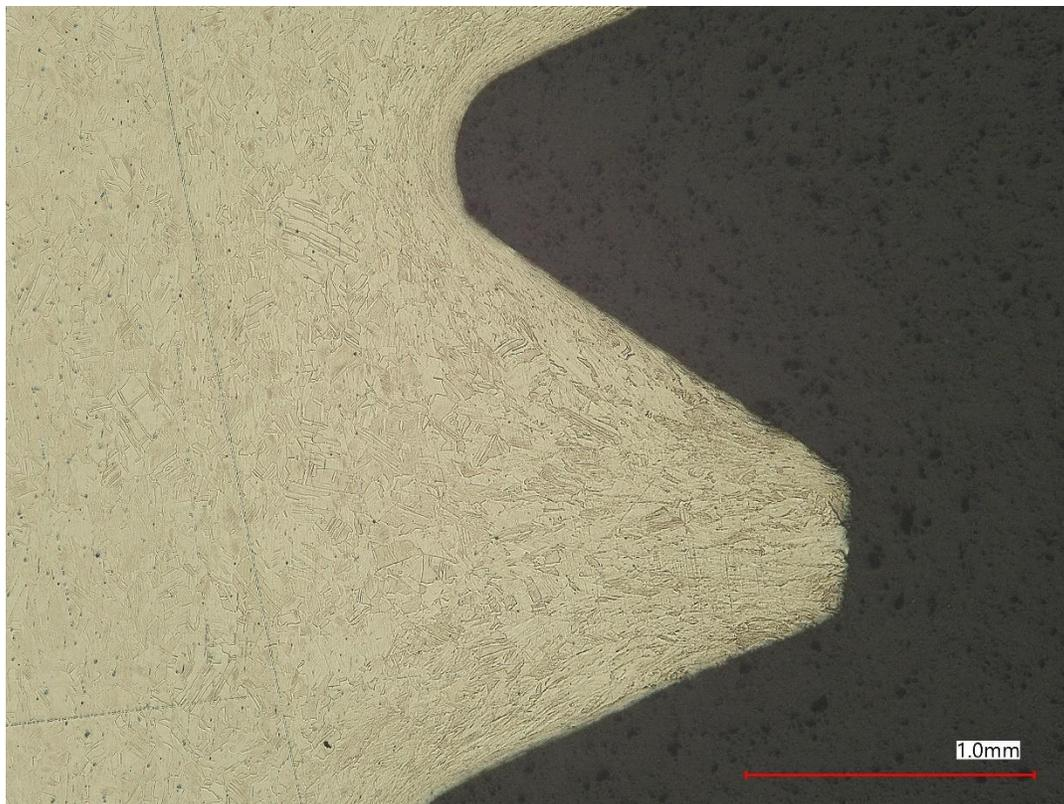
**FIGURE 64. MICROSTRUCTURE OF THREADS, BOLT O1**
