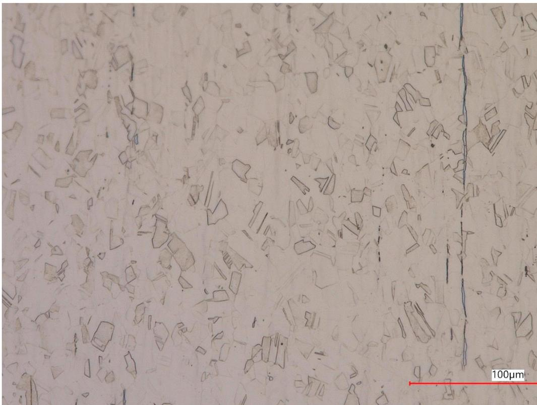
**FIGURE 62. CORE MICROSTRUCTURE OF BOLT C5**
