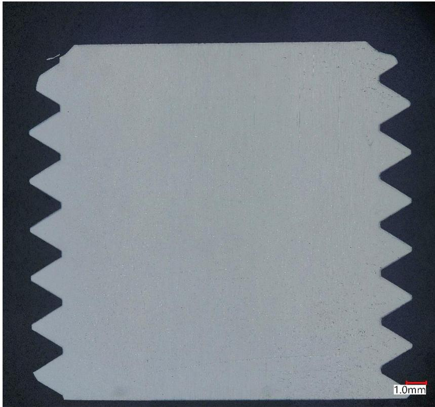
**FIGURE 69. GENERAL IMAGE OF BOLT R1 IN AS-POLISHED CONDITION**
