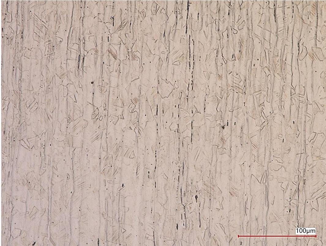
**FIGURE 83. CORE MICROSTRUCTURE OF BOLT R4**
