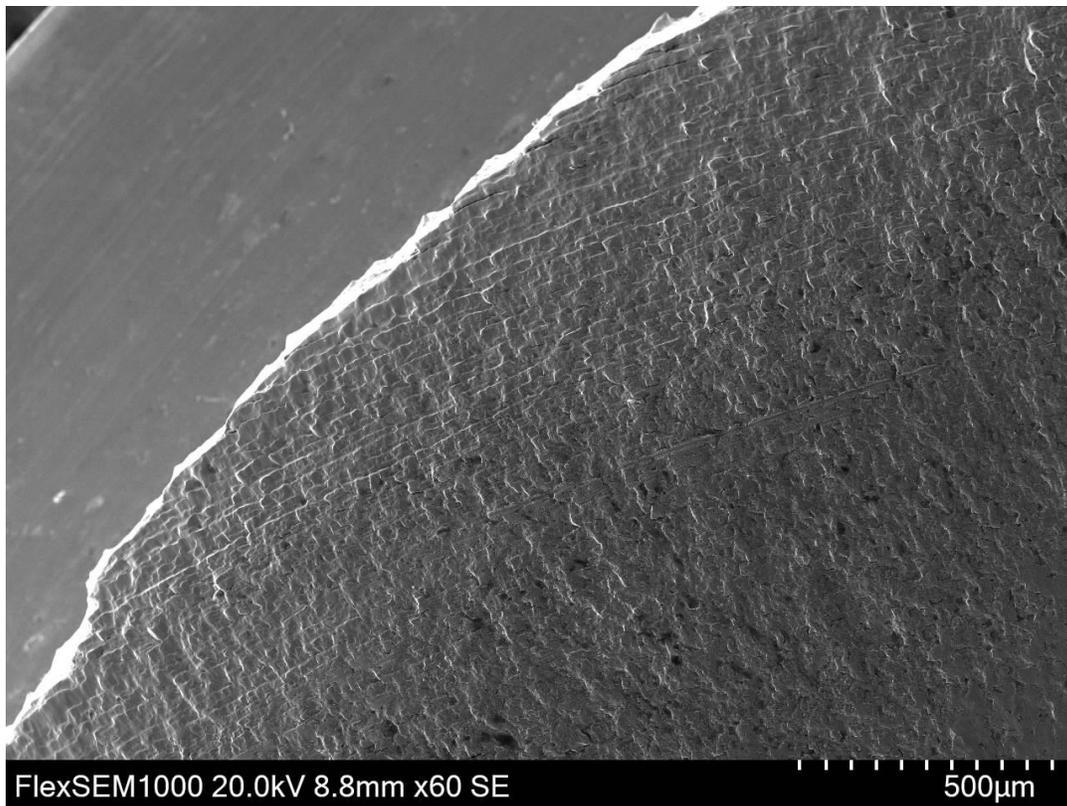
**FIGURE 37. BEACH MARKS AT 12 O'CLOCK REGION, BOLT C2**
