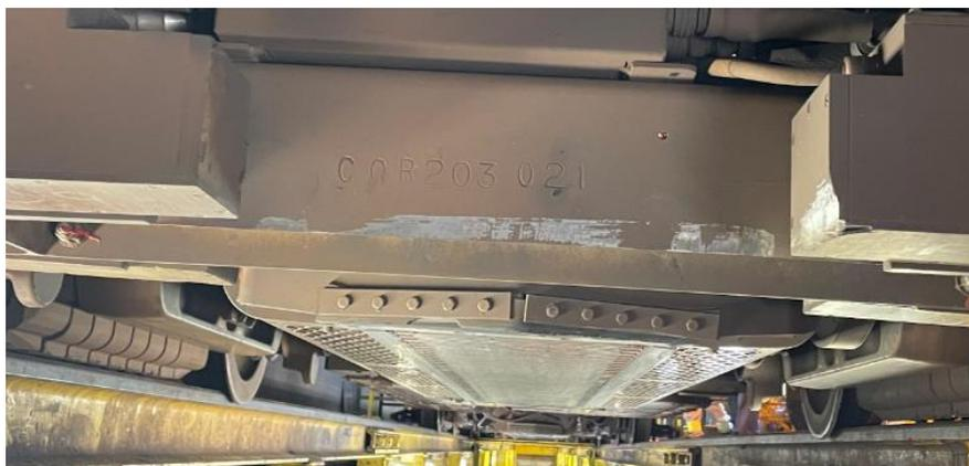
*Figure 6: Leading Edge Damage to Antenna Bridge on car 3009*
