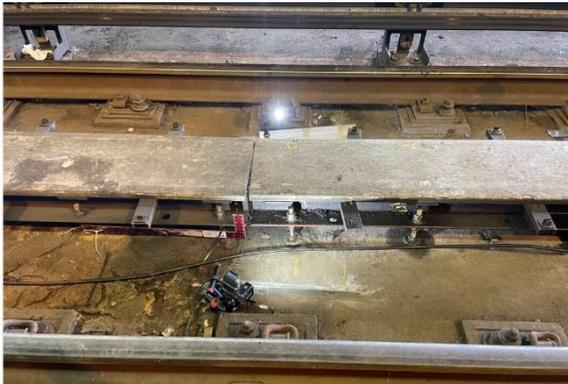
Figure 28: Go Pro Set Up on either side of the Reaction Rail
