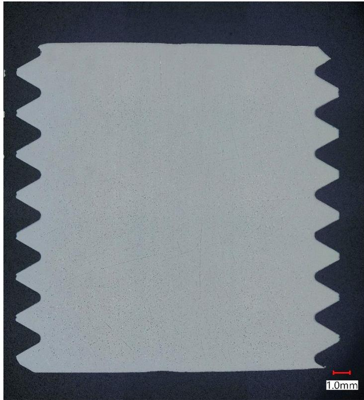
**FIGURE 63. GENERAL IMAGE OF BOLT O1 IN AS-POLISHED CONDITION**
