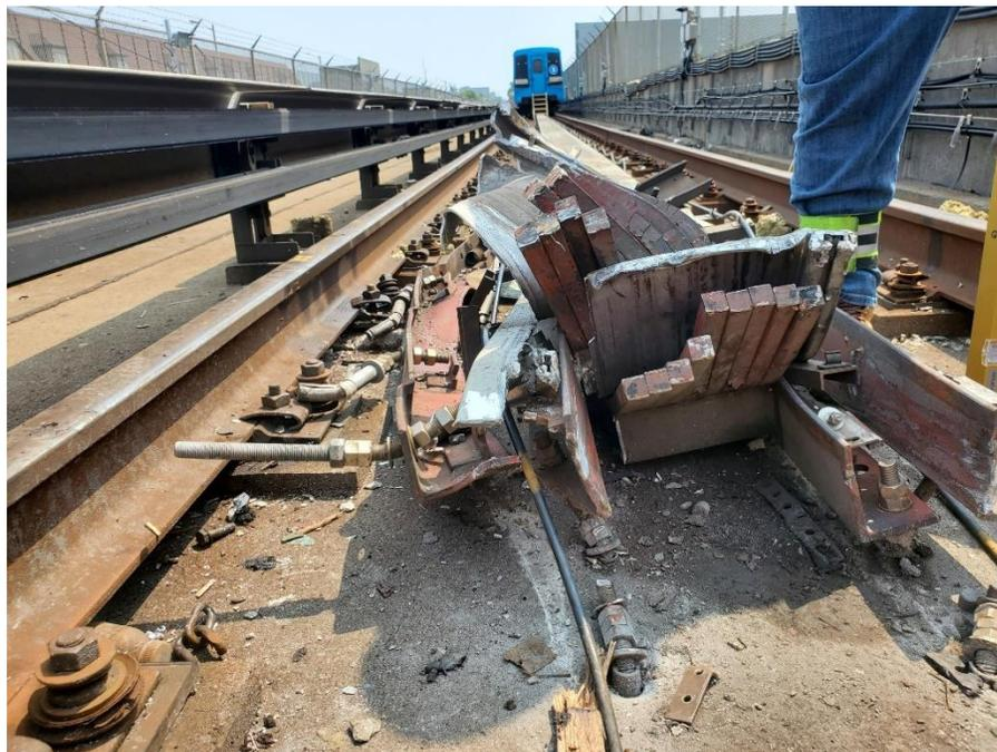
*Figure 11: Section of reaction rail which came into contact with the linear induction motor.*
