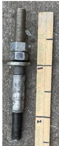
Figure 23: Partial Anchor Assembly Found at Derailment Site
