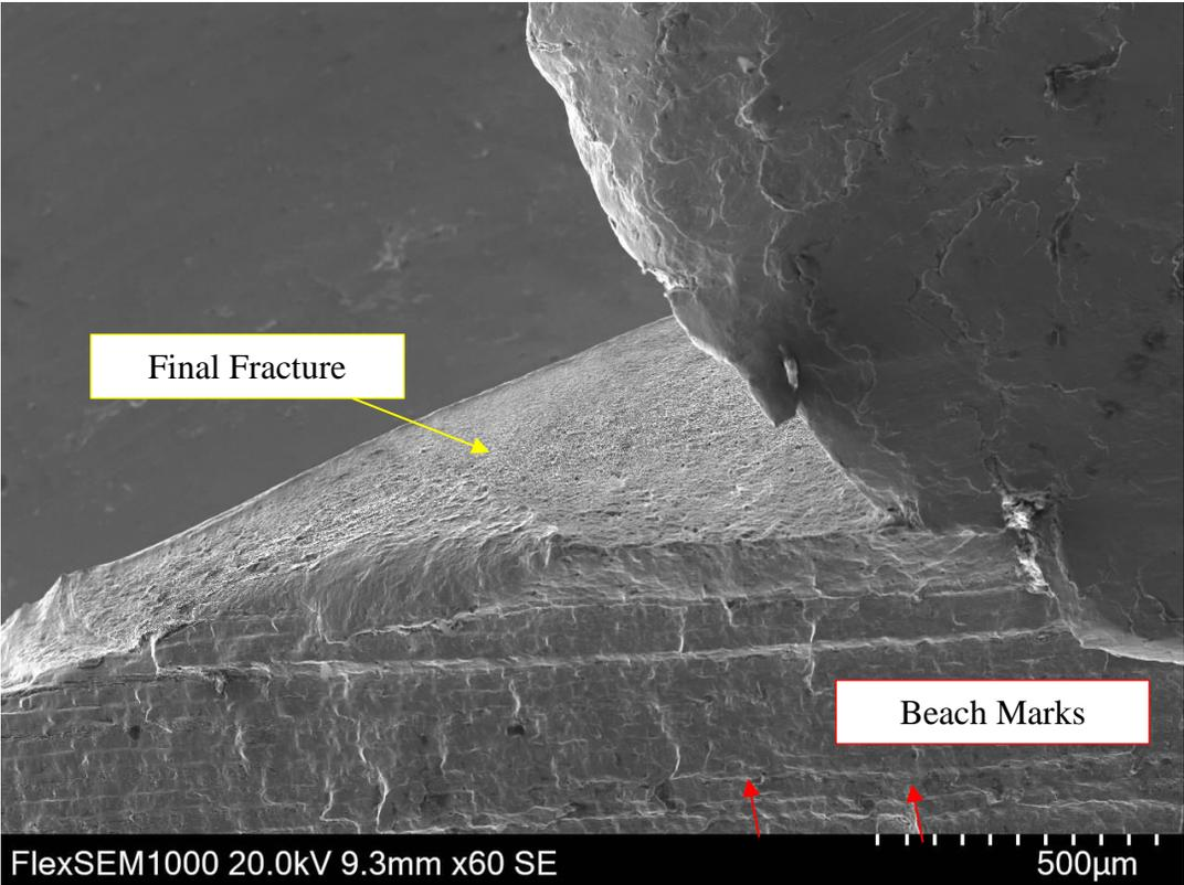
**FIGURE 43. TOP END OF THE FRACTURE SURFACE (SEE FIGURE 19), BOLT C2**
