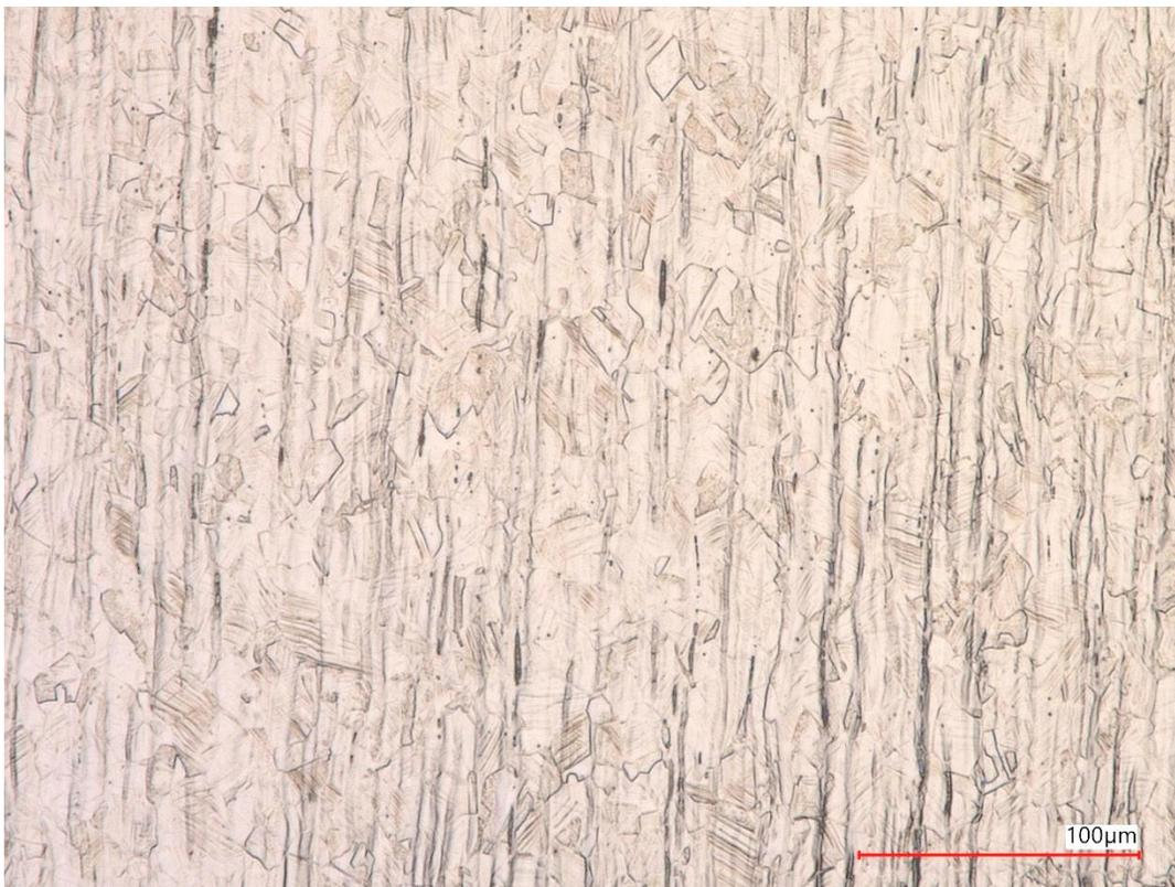
**FIGURE 76. CORE MICROSTRUCTURE OF BOLT R2**
