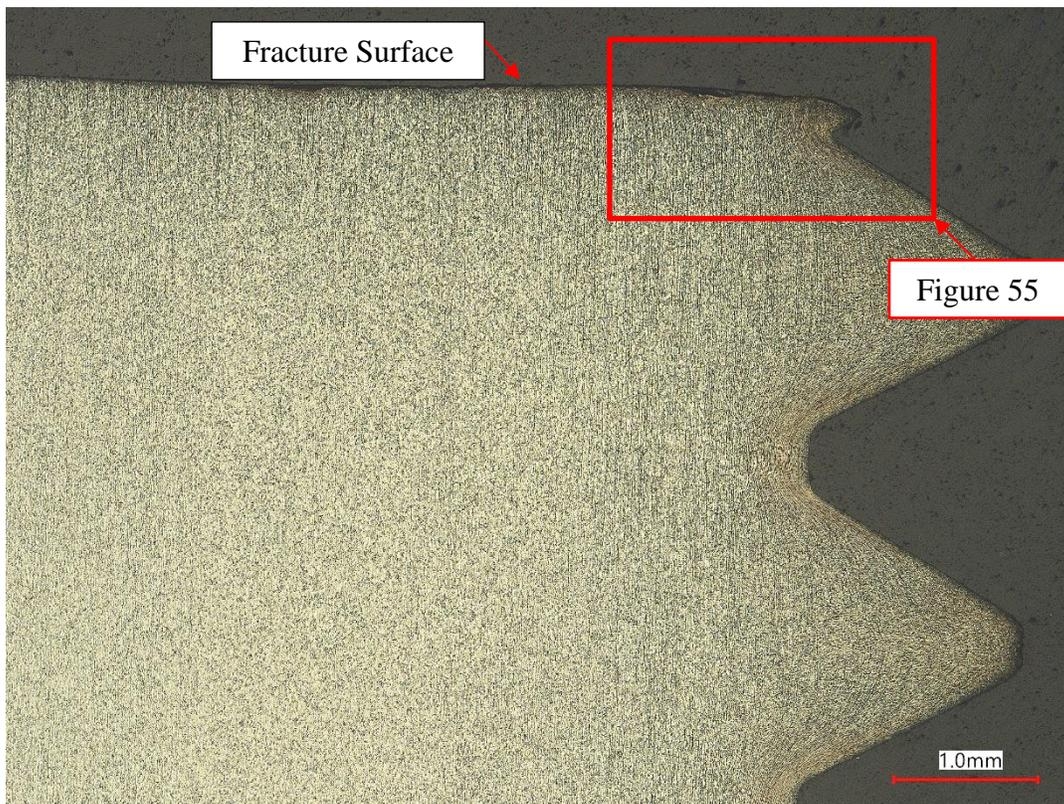
**FIGURE 54. LOW MAGNIFICATION OF THREADS CLOSE TO CRACK INITIATION AREA AT 6 O'CLOCK REGION, BOLT C2**
