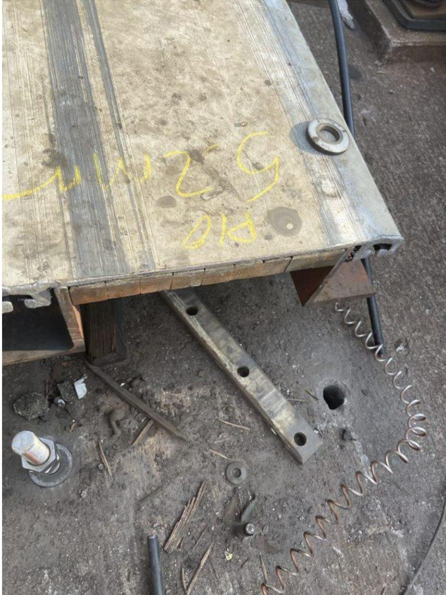
*Figure 7: Anchor Bolts zero (0) and one (1) at point of impact. Top cap abrasion*
