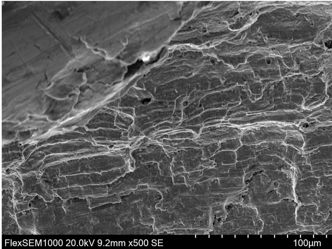
**FIGURE 38. CLOSE VIEW OF THE BEACH MARKS AT 12 O'CLOCK REGION, BOLT C2**
