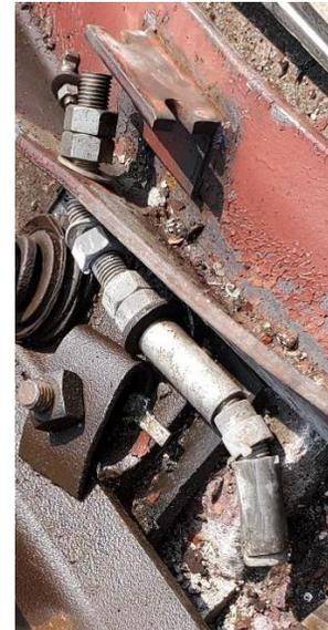
Figure 24: Anchor Assembly (pullout failure)
