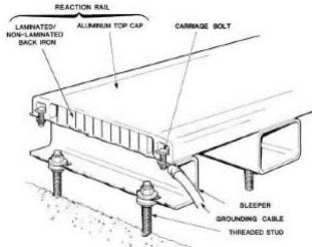
Figure 13: Typical Reaction Rail
