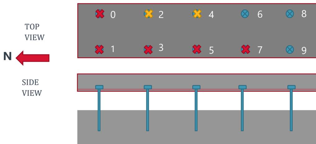
Figure 32: Bolt Failure configuration diagram. Red represents confirmed failed anchor bolts, and yellow represents suspected loose anchor bolts
