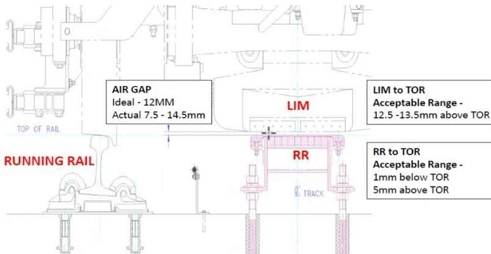
Figure 14: Reaction Rail to Top of Running Rail
