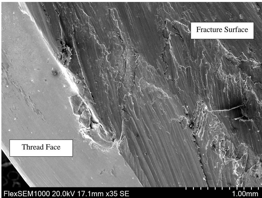
**FIGURE 49. FRACTURE SURFACE AND THREAD FACE, BOLT C5**
