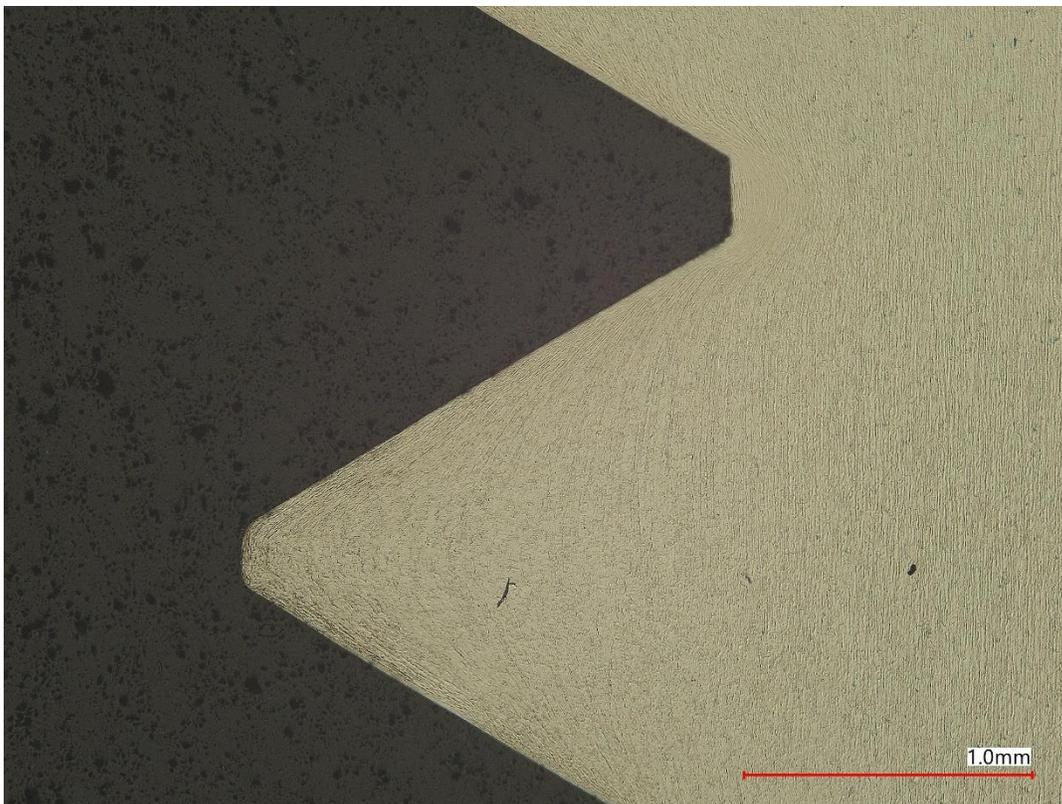
**FIGURE 78. FLOW LINES ON THREADS, BOLT R3**
