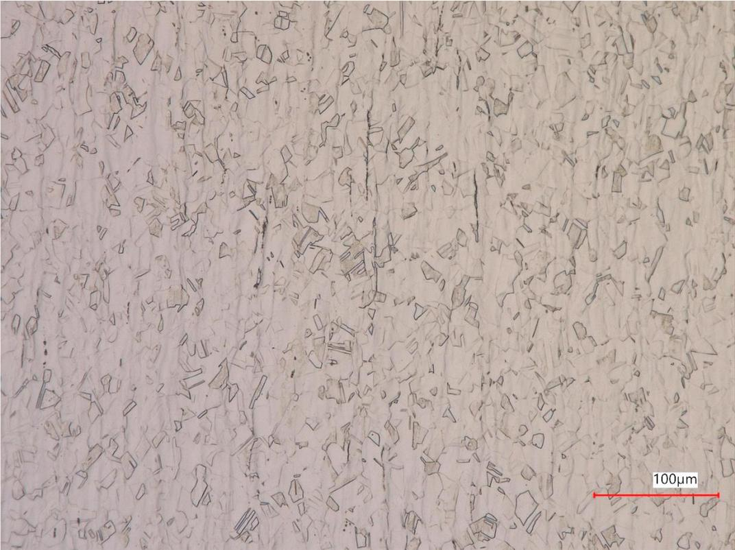
**FIGURE 59. CORE MICROSTRUCTURE, BOLT C2**
