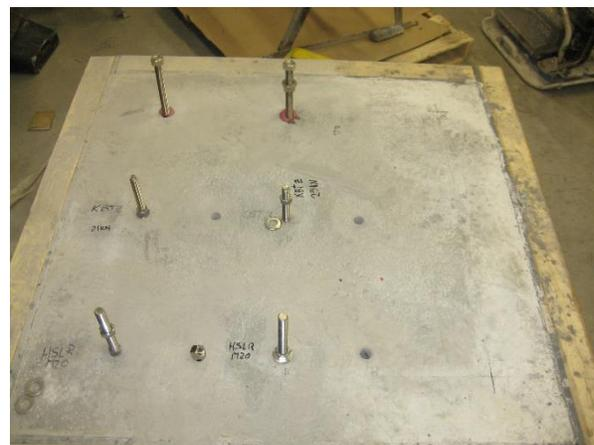
Figure 26: Post-Installed Anchor Test
