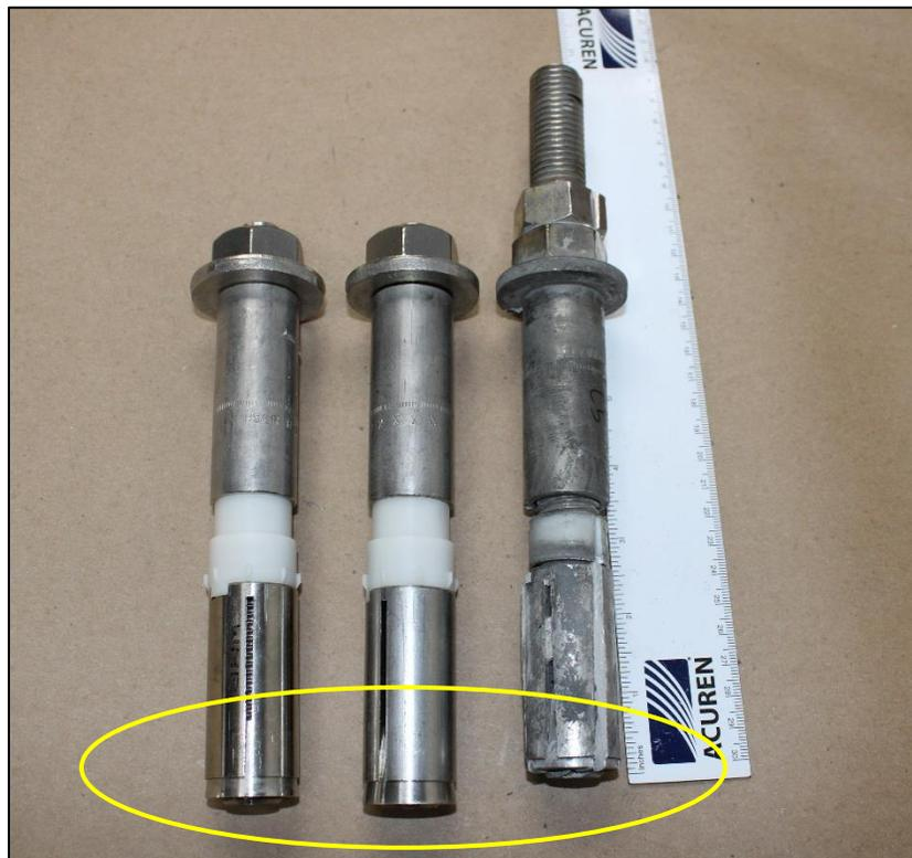
**FIGURE 10. PHOTOS DISPLAYING THE SLIGHT CURVE OBSERVED IN BOLT C5 COMPARED TO THE ORIGINAL BOLTS. THE INSERTS AT THE BOTTOM OF THE ANCHOR FIXTURING WAS DIFFERENT BETWEEN THE ORIGINAL BOLTS AND BOLT C5.**
