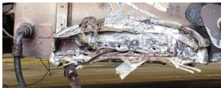
*Figure 7: Leading Edge Damage to LIM on car 3001*
