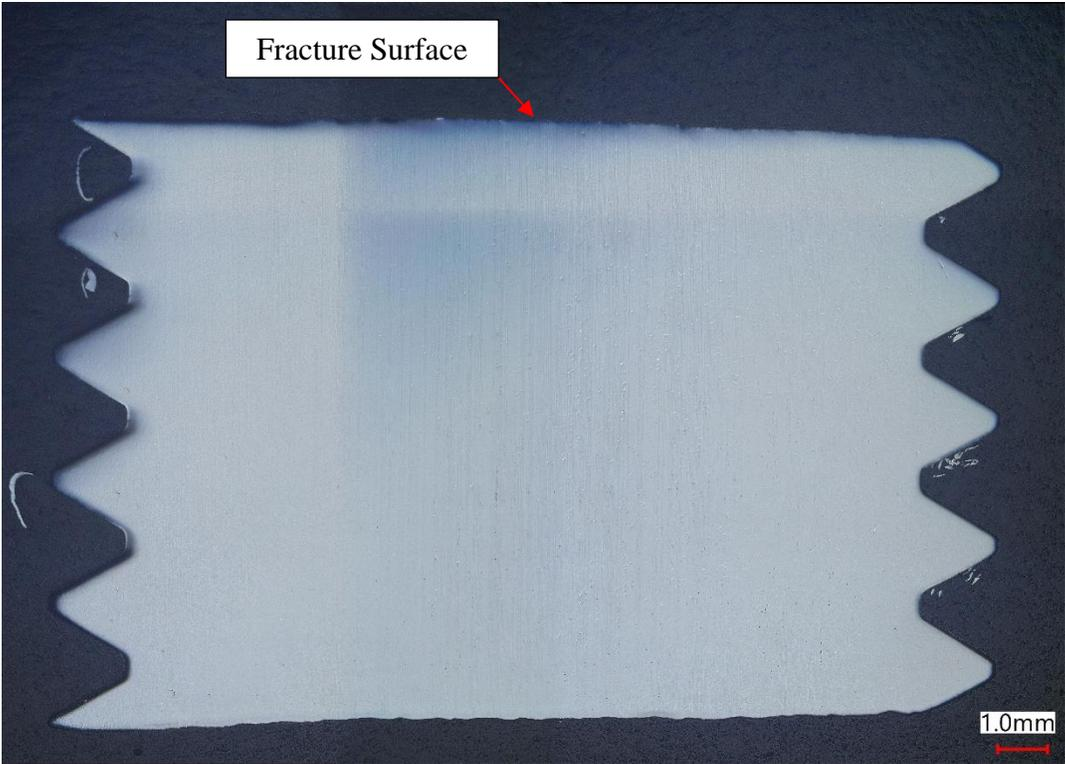
**FIGURE 60. GENERAL IMAGE OF BOLT C5 IN AS-POLISHED CONDITION**
