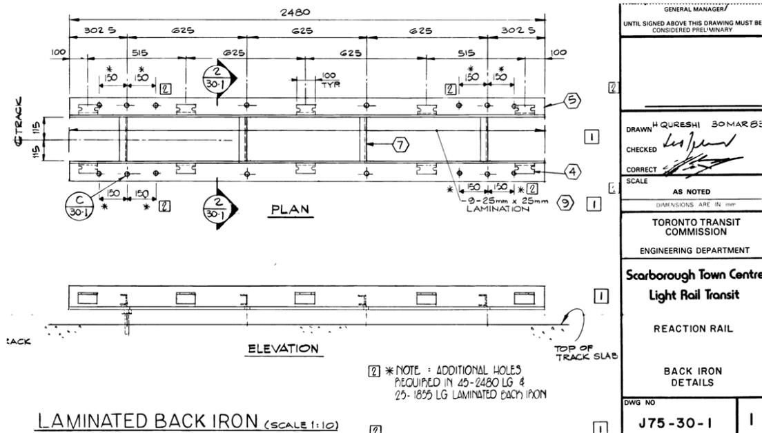
Figure 18: Typical Reaction Drawing - Plan and Elevation
