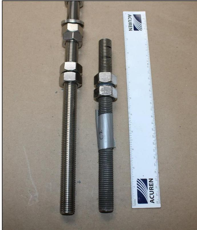
**FIGURE 8. PHOTO DISPLAYING A SLIGHT CURVE IN BOLT C2 UPON INITIAL EXAMINATION.**
