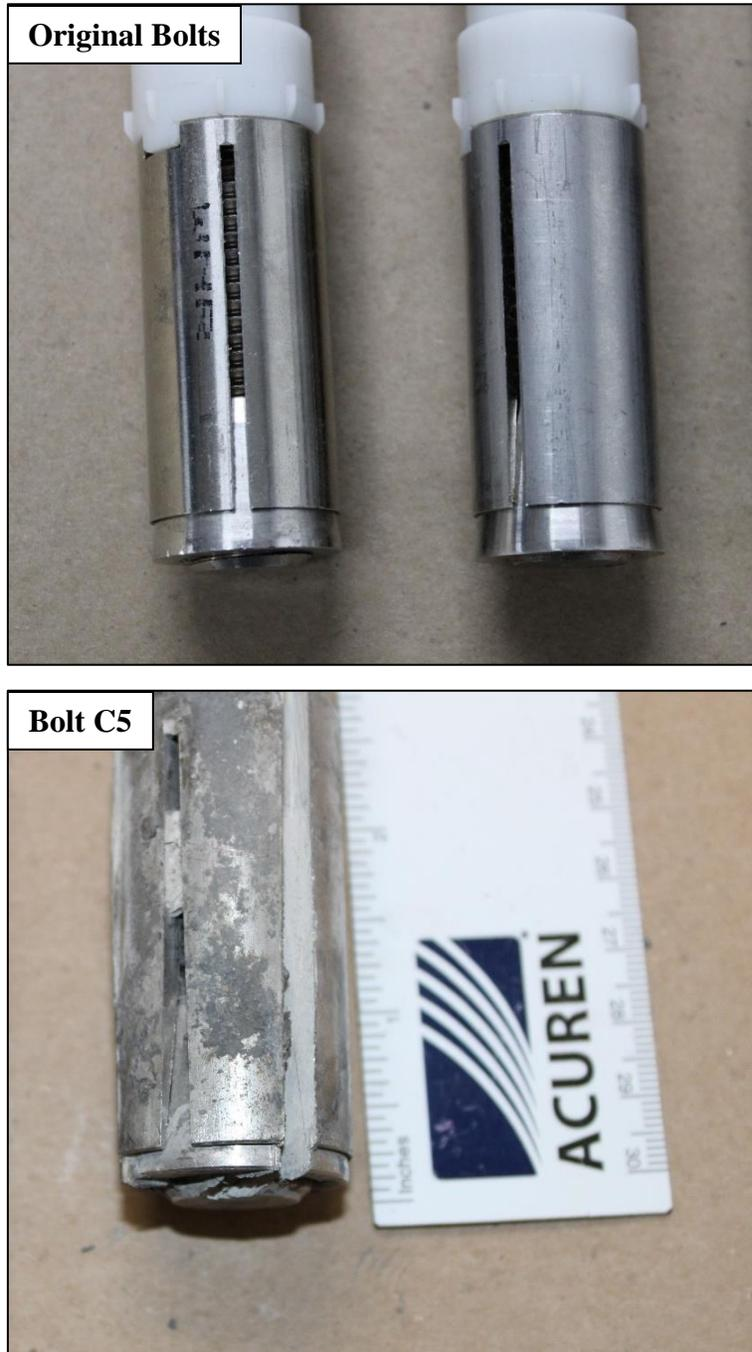
**FIGURE 11. PHOTOS SHOWING THE BOTTOM OF THE ANCHOR FIXTURING ON THE ORIGINAL BOLTS AND BOLT C5.**
