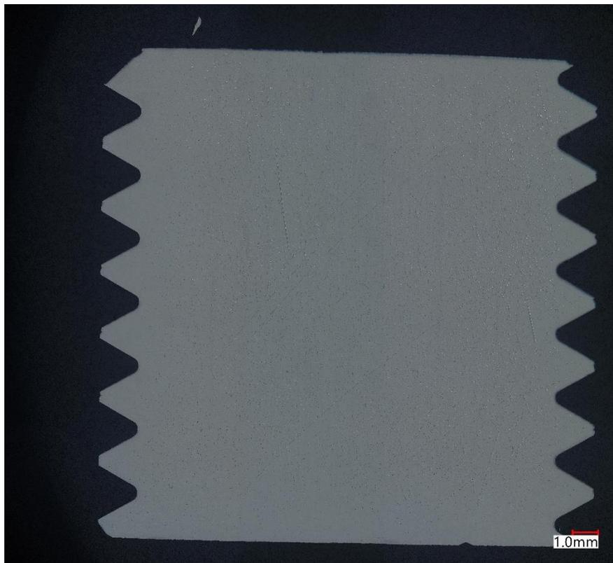
**FIGURE 66. GENERAL IMAGE OF BOLT O2 IN AS-POLISHED CONDITION**
