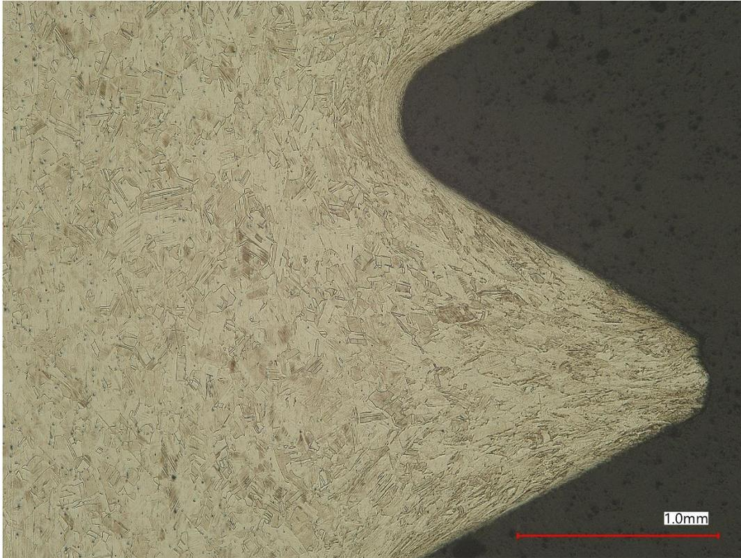
**FIGURE 67. MICROSTRUCTURE OF THREADS, BOLT O2**
