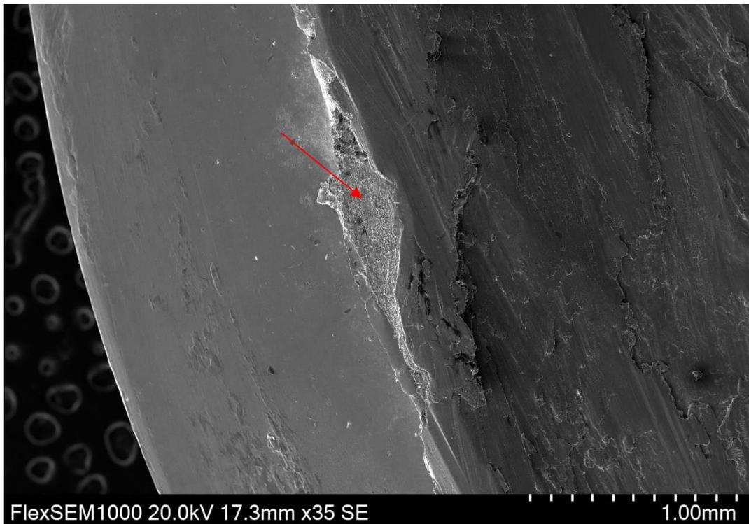
**FIGURE 51. POCKET OF THE THREAD FACE – FRACTURE SURFACE BORDER, BOLT C5**
