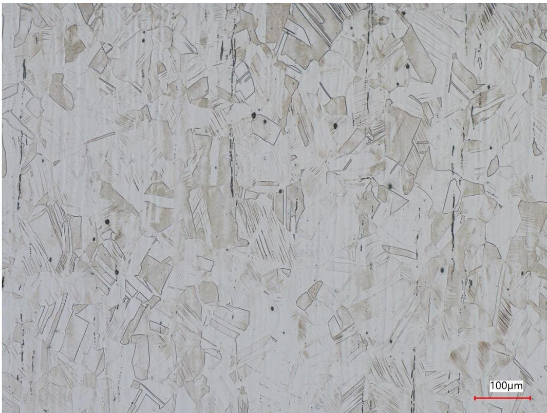
**FIGURE 68. CORE MICROSTRUCTURE OF BOLT O2**
