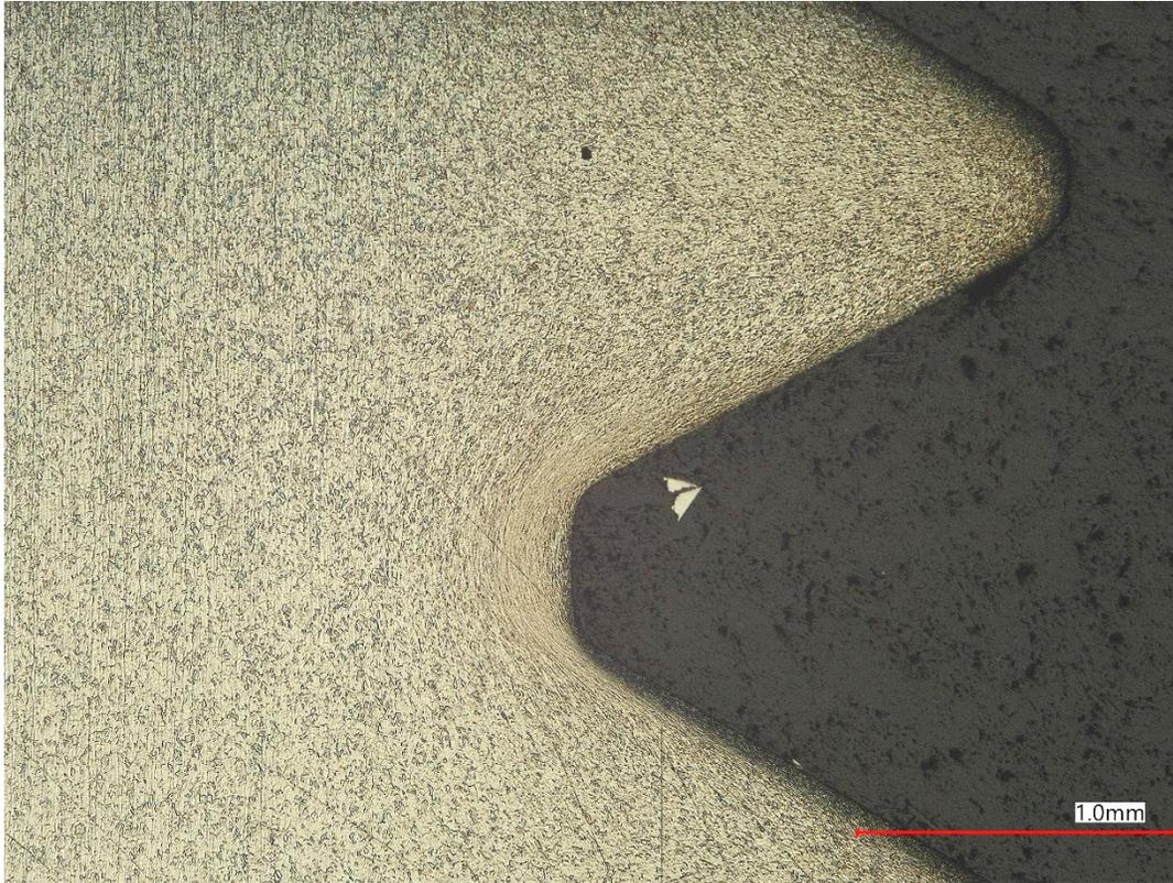
**FIGURE 61. FLOW LINES ON THE THREADS, BOLT C5**
