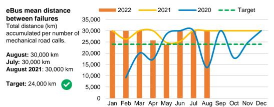
Hybrid bus mean3distance between failures3Total distance (km)3accumulated per number of<br/>mechanical road calls.2
