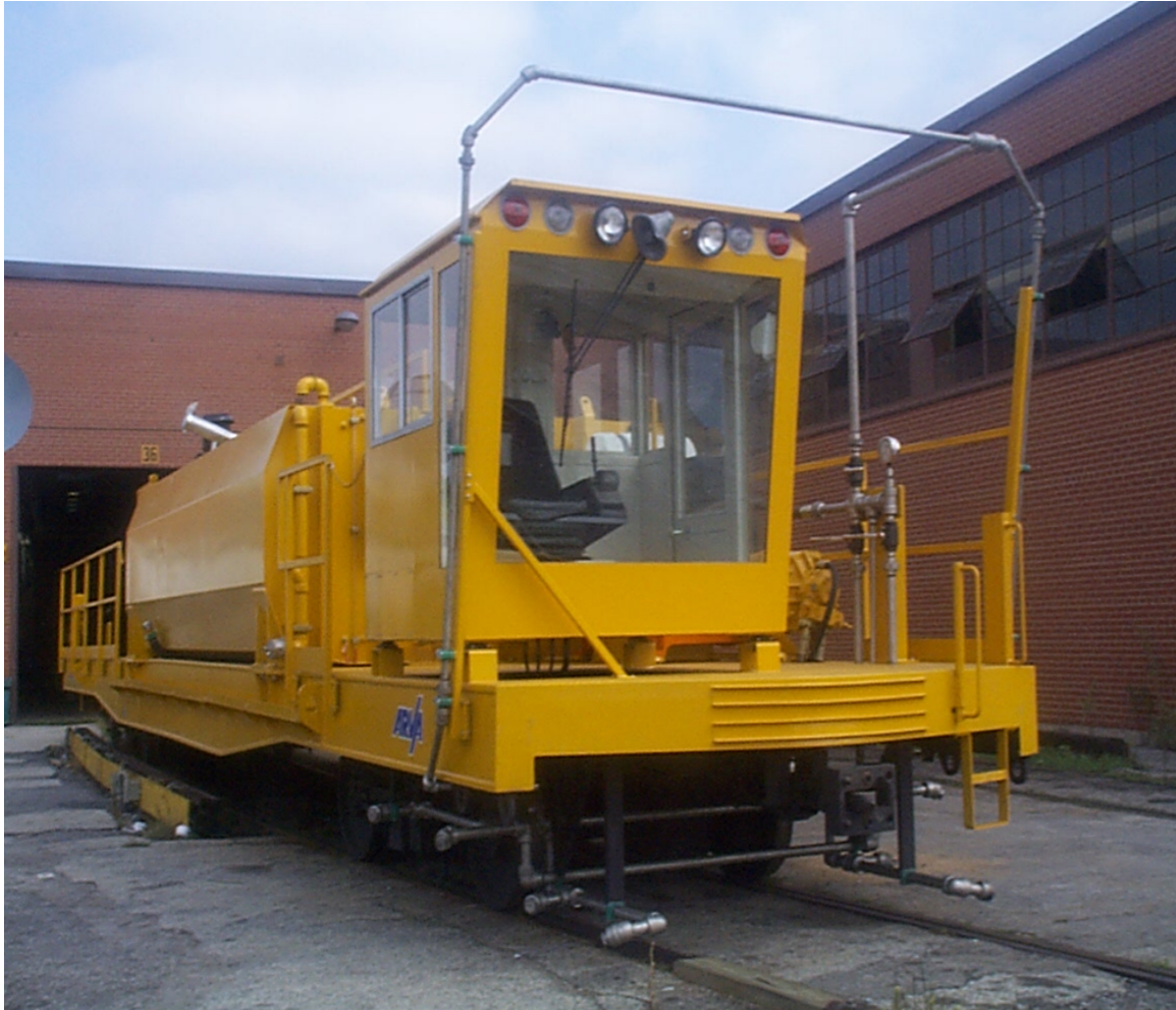
RT-17: Tunnel Washer Work Car
