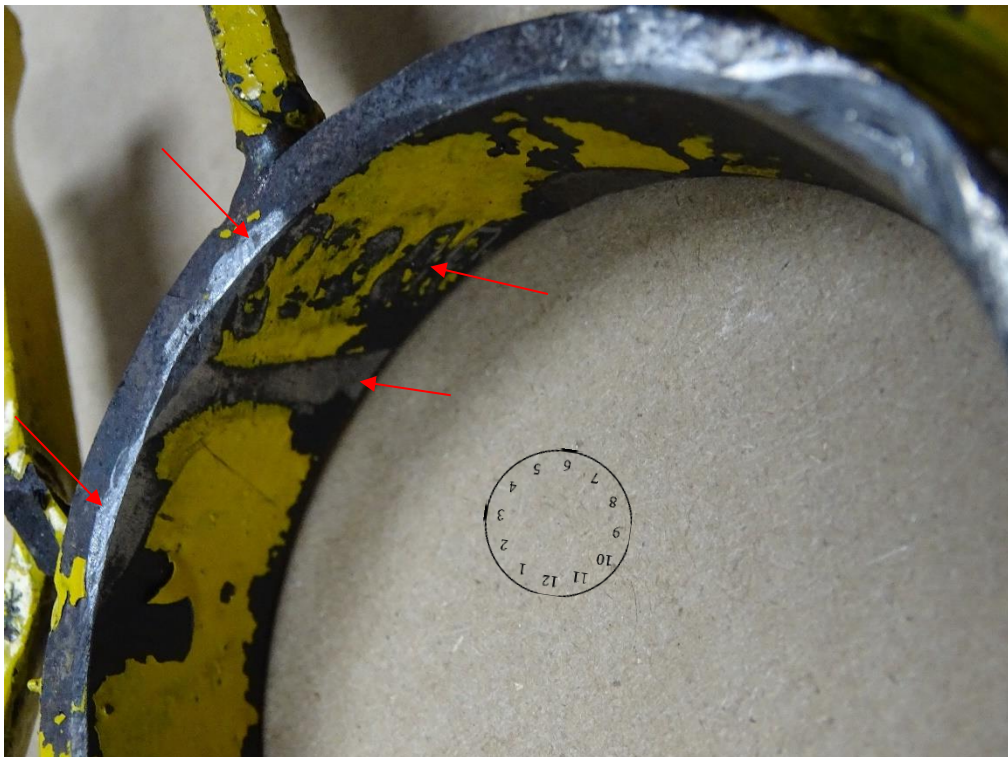
FIGURE 14. EVIDENCE OF RUBBING AT 4 AND 5 O'CLOCK
