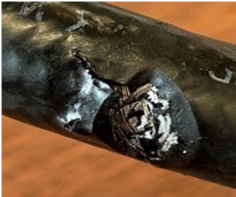
Figure 12 - Abrasion on the hose
