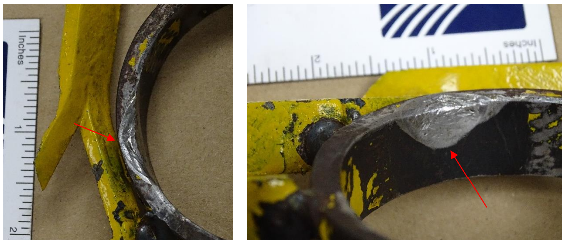
FIGURE 12. DEFORMATION OBSERVED ON THE RING AT AROUND 8 O'CLOCK LOCATION
