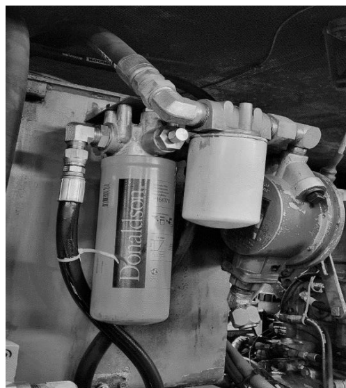
Figure 5 - RT7 Hydraulic Filter and Filter Mounting Housing, New Configuration (Current)
