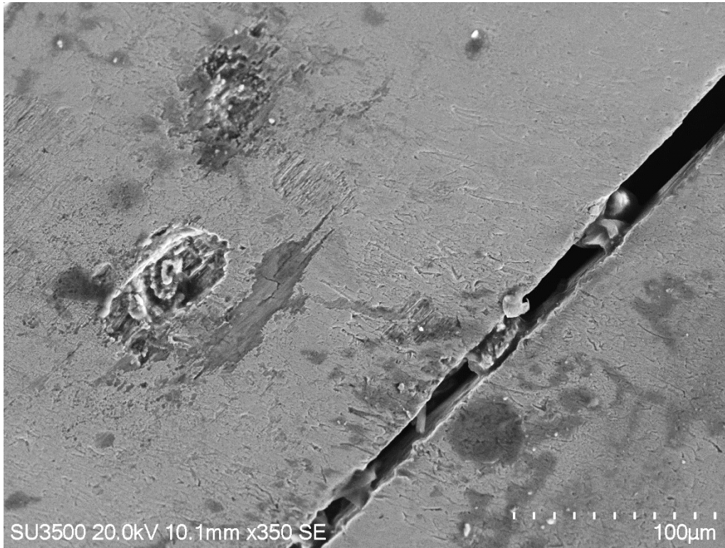
FIGURE 30. WEAR MARKS ON THE WIRE STRANDS IN THE DAMAGED AREA 2
