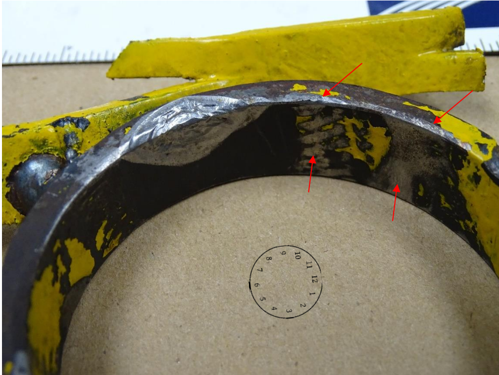
FIGURE 13. EVIDENCE OF RUBBING AT 10 AND 11 O'CLOCK
