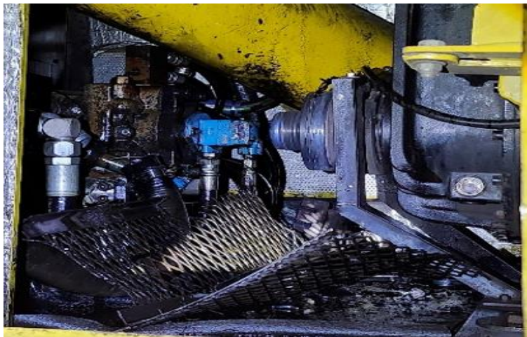
Figure 20 - RT84 engine compartment with broken drive shaft and damaged shaft guard
