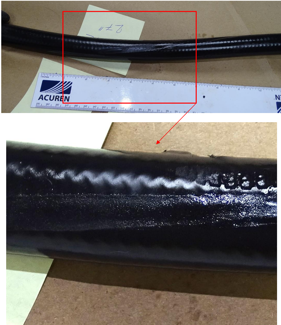
FIGURE 9. AREA #4 – SHOWING RUBBING/DAMAGE ON COVER
