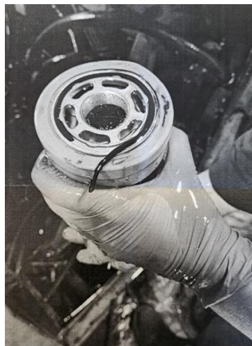
Figure 3 - RT17 Close-up view of failed hydraulic filter O-ring
