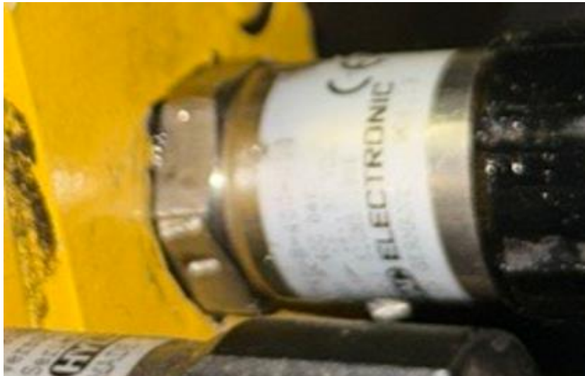
Figure 25 - Marks on RT41 pressure sensor
