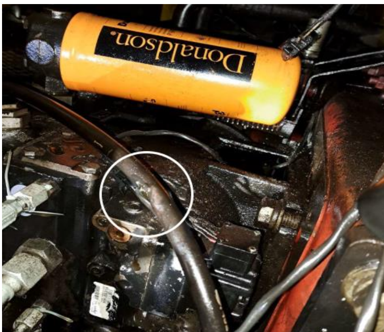
Figure 1 - Ruptured hose on RT56 on Jan. 14
