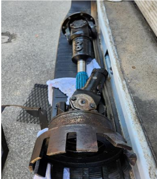
Figure 18 - RT84 clutch housing with broken driveshaft
