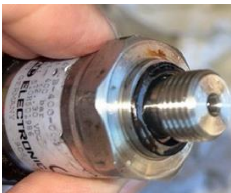
Figure 23 - RT41 Pressure Sensor with O-ring
