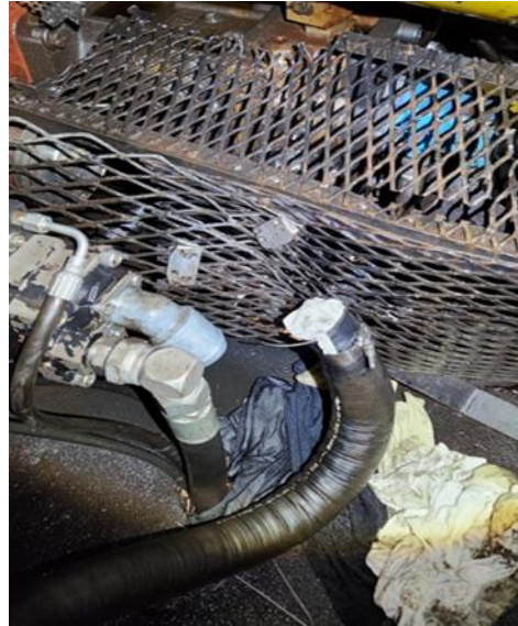
Figure 19 - RT84 severed hydraulic hose
