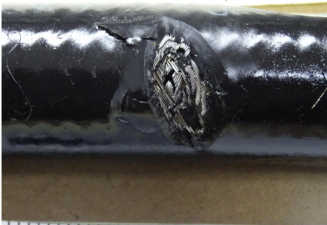
FIGURE 8. AREA 3 – SHOWING TEARING/CRACKS IN THE COVER, WIRES ARE EVIDENT AND A HOLE IS OBSERVED
