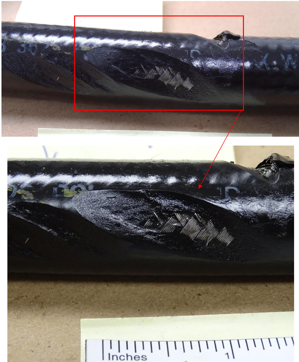
FIGURE 7. AREA #2 – SHOWING DAMAGE ON THE COVER, THE REINFORCEMENT WAS EXPOSED
