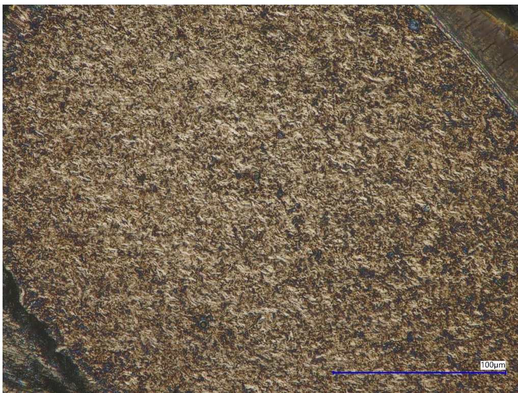
FIGURE 52. MICROSTRUCTURE OF WIRE STRANDS
