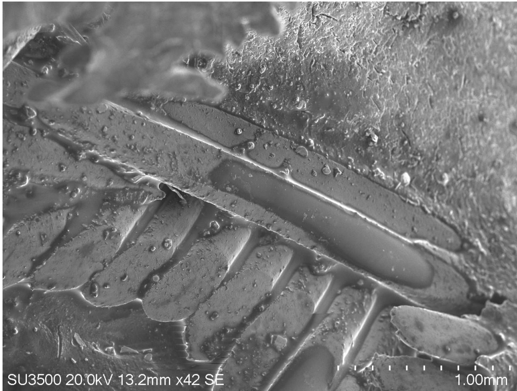
FIGURE 40. EXPOSED WIRE STRANDS IN DAMAGED AREA 3
