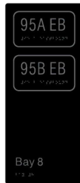
Typical Tactile & Braille (T&B) bay number and route identification sign
