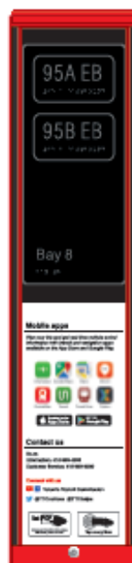
Typical bay numbering stop marker w/ Infopost frame and insert and applied T&B sign
