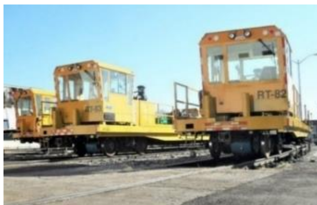
Figure 4-9: Rail maintenance vehicles
