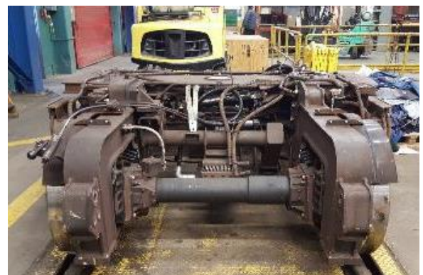
Figure 4-5: Completed overhaul of TR non-powered truck.
