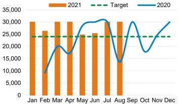
Hvbrid bus mean distance between failures Total distance (km) accumulated per number of mechanical road calls.
