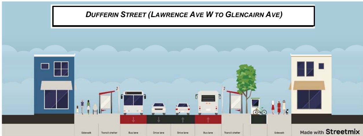
FIGURE 4: DUFFERIN STREET – 2 GENERAL PURPOSE LANE + 2 BUS LANE CROSS-SECTION
