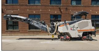
A production concrete milling unit
