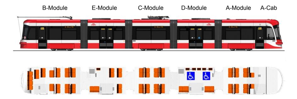
• Within the D-Module underframe is an electrically powered ramp
