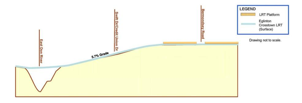
Exhibit 4 Cross-Section Showing Potential LRT Stop at Swift/ Credit Union (Not Recommended)
