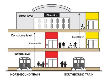
Provides a barrier-free path to all levels of the station including installation of:
