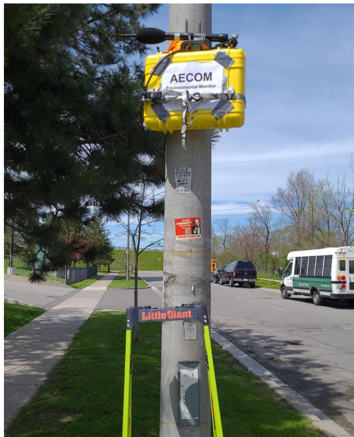
Figure 2: Example Noise Monitor Setup
